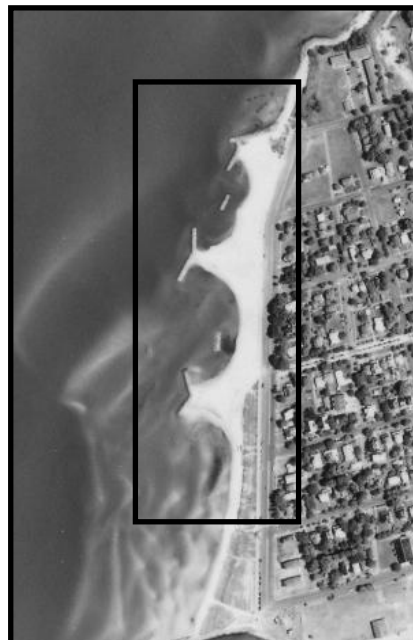
Figure CCPB1. Aerial photo of the breakwater at Cape Charles Public Beach, VA.
