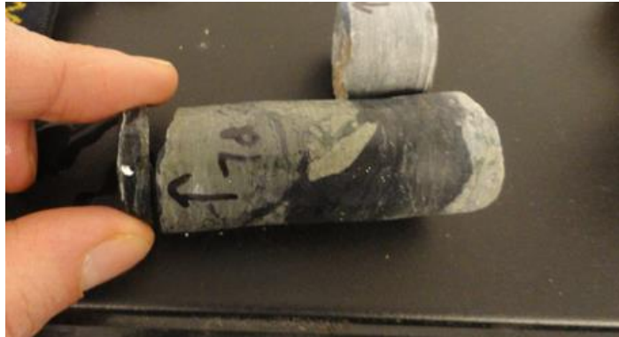
Figure 9: Sample of drill core from the lawsonite-albite facies showing mafic block (green) and matrix (black). Part of the block has broken off and was surrounded by matrix.
