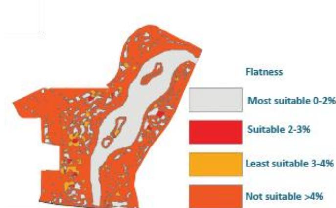
**Figure 3.32: Slope Suitability Model**
