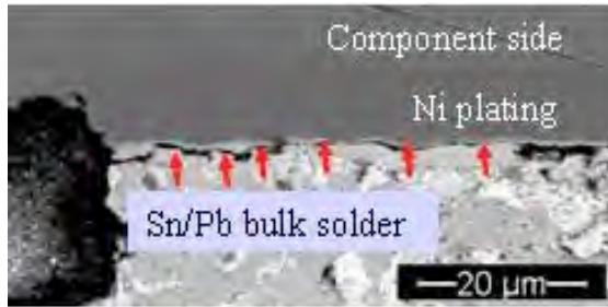
Figure 5-3: Fracture in the IMC layer on the package side of the solder [86][85]
