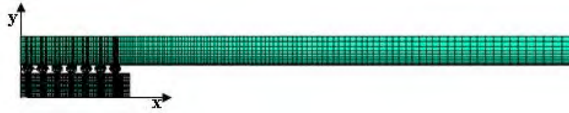
Figure 6-7: 2D model of PWA with symmetric boundary conditions
