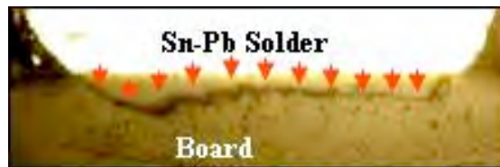
Figure 3-9: Crack in FR4 under the solder ball.
