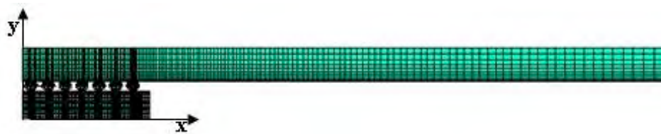
Figure 5-4: 2D model of PWA with symmetric boundary conditions
