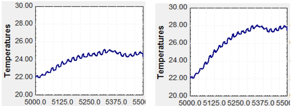
**Figure 18: 3-Week Attic Temperature: White Roof (L) and Black Roof (R)**
