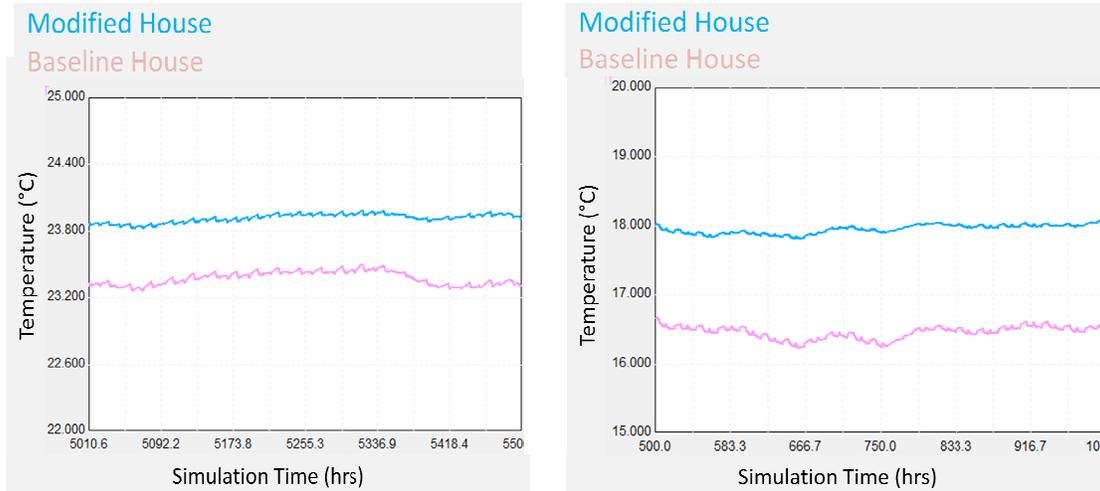
**Figure 16: Basement Temperature Differences (C) – Summer (L) and Winter (R). Please note difference of scale.**
