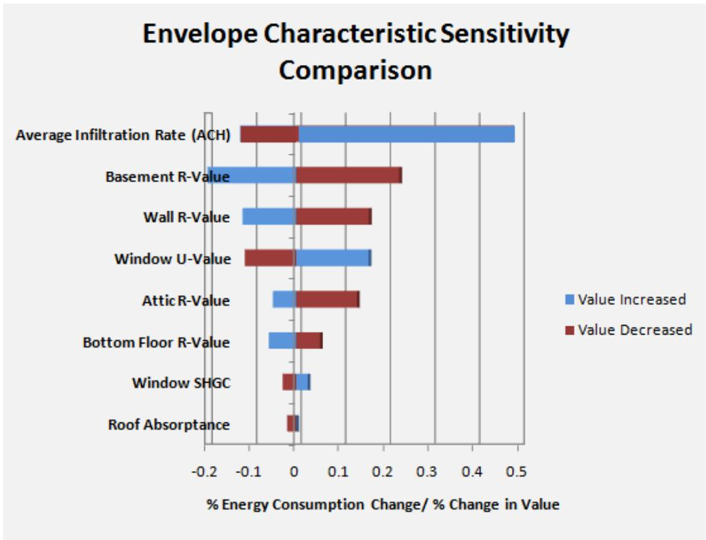
Figure 19: Envelope Characteristic Sensitivity Comparison
