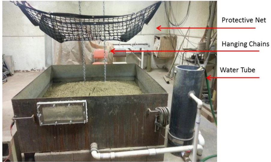
Figure 2.9: Test bed showing hanging chains, net, and water tube
