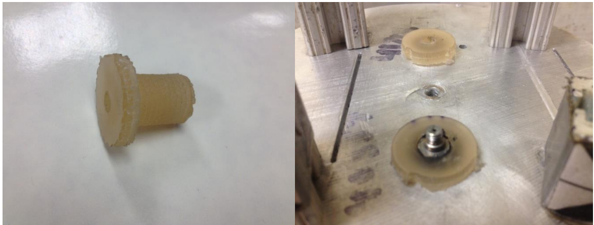
Figure 2.4: Rubber pad removed from plate (left) and two rubber pads inserted into a test plate (right), one containing an accelerometer and one empty
