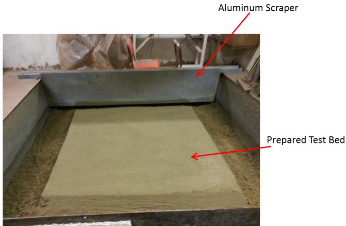
Figure 2.16: Prepared test bed, showing aluminum scraper
