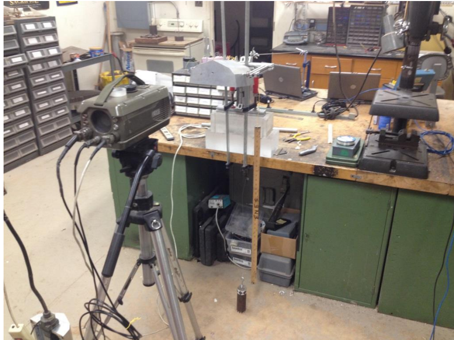
Figure 2.15: Phantom v12.1 tracking rotational velocity of plate
