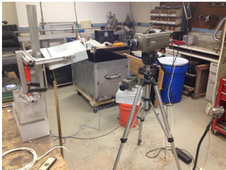
Figure 2.14: Phantom v12.1 cameras tracking both hanging mass (lower camera) and plate rotation (higher camera)
