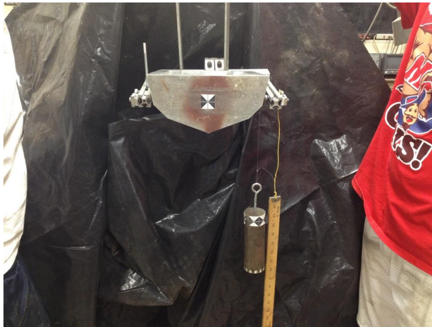
Figure 2.13: V-shaped bottom with hanging mass and tracking target attached
