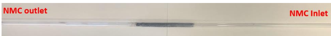
Figure 3.6. Inner tube of ACWR after 6 hours of reaction. (Reaction condition: 0.48 L h -1 gas flow with CH 4 :Ar ratio = 7, 101.325 kPa pressure, 0.2 g Fe/SiO 2 catalyst in ACWR, Fe concentration = 0.075 wt%; Fuel combustion: 165 L h -1 gas flow with CH 4 :Air ratio = 0.1, 101.325 kPa pressure, 0.1 g Pt/Al 2 O 3 catalyst, Pt concentration = 1.0 wt%)
