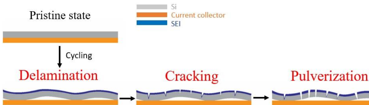
Figure 1. 2: Schematic of mechanical failure modes of c-Si electrodes
