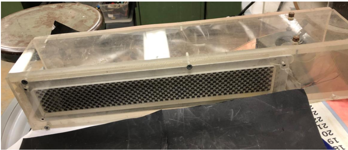
Figure 9: LED array for analyzing crack development after loading
