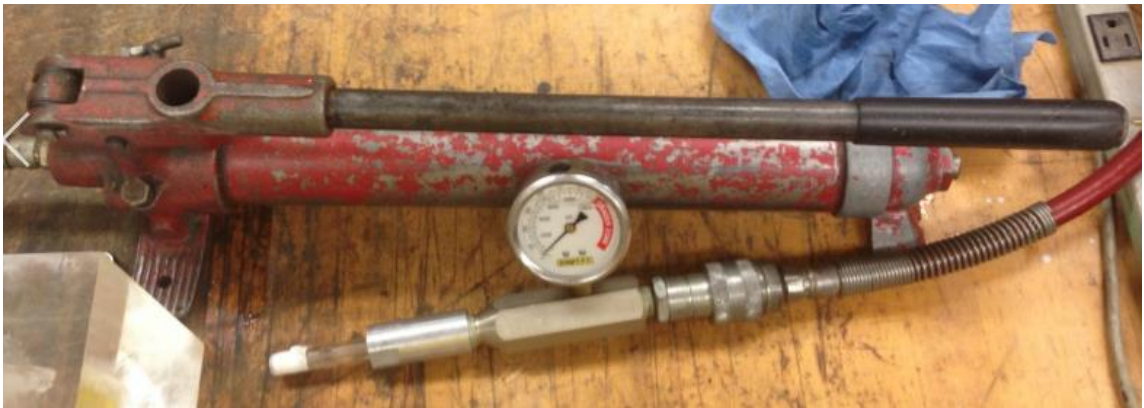
Figure 11: Hydraulic hand pump used for quasi-static loading
