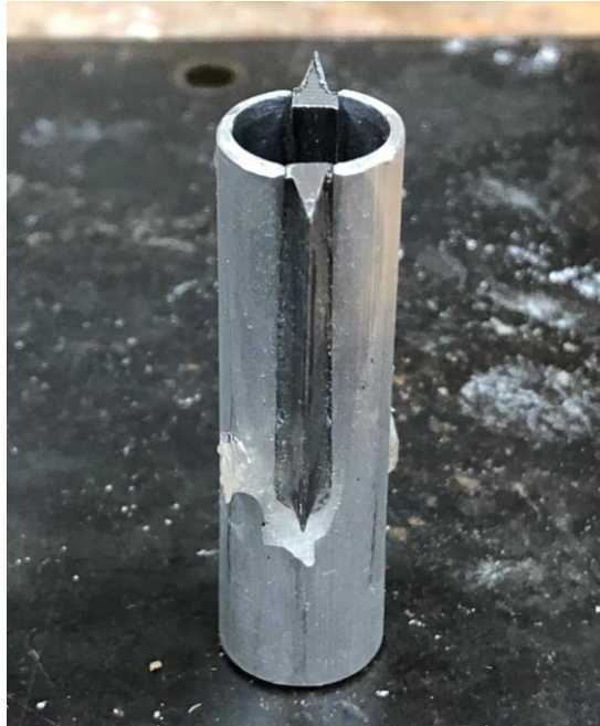
Figure 15: Aluminum rod and steel wedges subassembly
