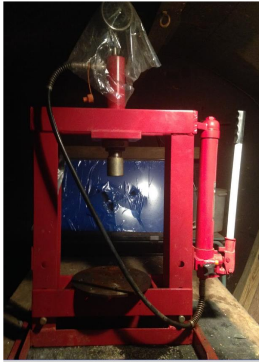
Figure 10: Hydraulic hand press used to simulate in situ stress
