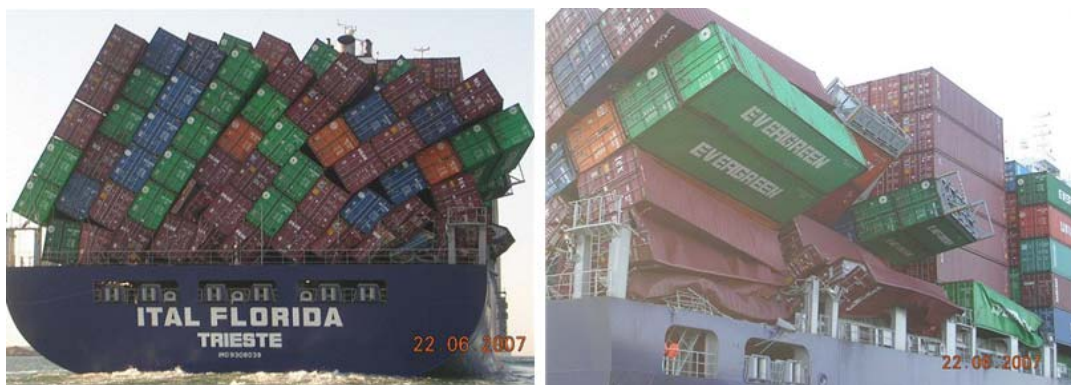
Figure 3.7: Damaged containers on Ital Florida ( www.cargolaw.com )
