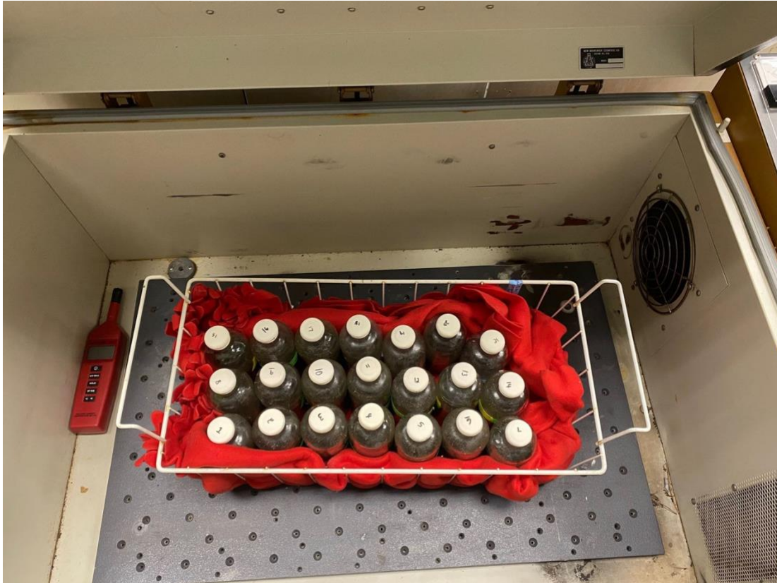
Figure 3.3: Example of a batch-scale reactor experiment setup using glass bottles, with rubber septa attached.
