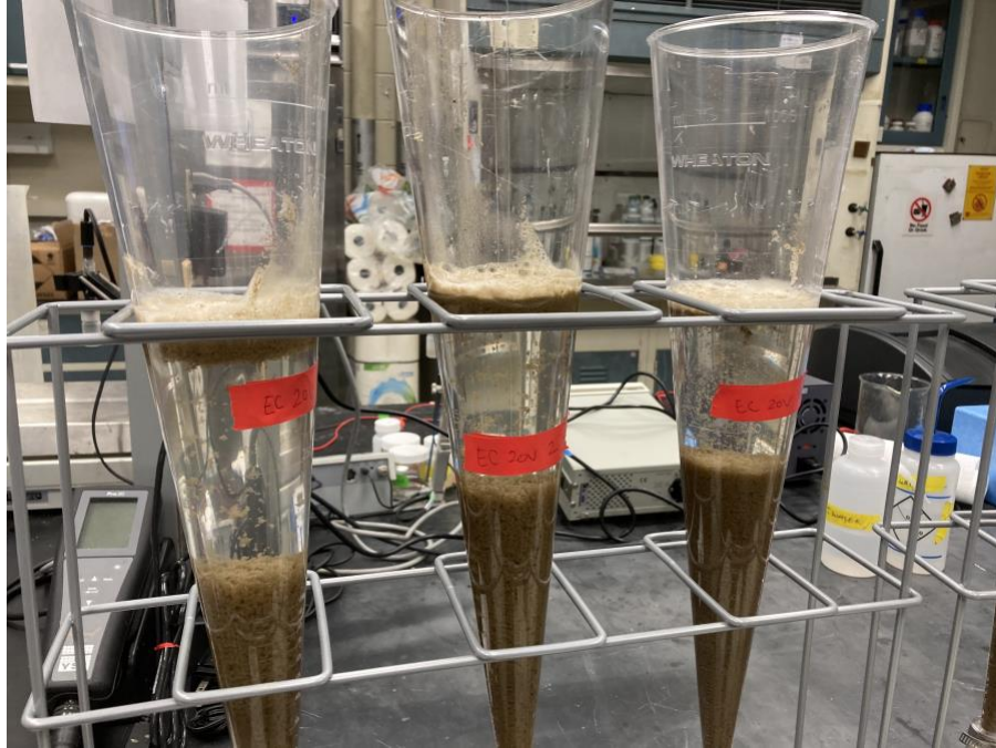
Figure 4.2: Imhoff settling cone setup during the coagulation dewatering experiment.
