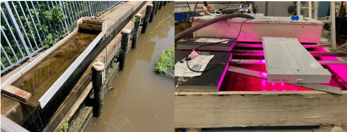
Figure 4.1: Algal turf scrubbers (ATS) unit 1 (left) and unit 2 (right) that were used to supply algae for the coagulation dewatering experiment.
