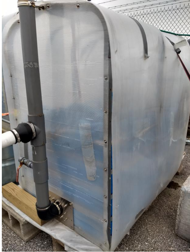
Figure 2.2: An anaerobic digester used at the Port of Baltimore Dundalk Terminal (Baltimore, MD, USA).
