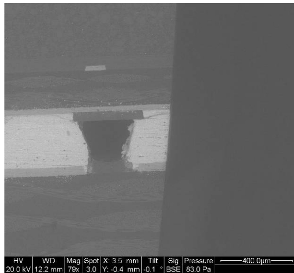
Figure 29. Cross section of corner SnPb solder ball, component U4, ball P1 BGA cross-section cornered
