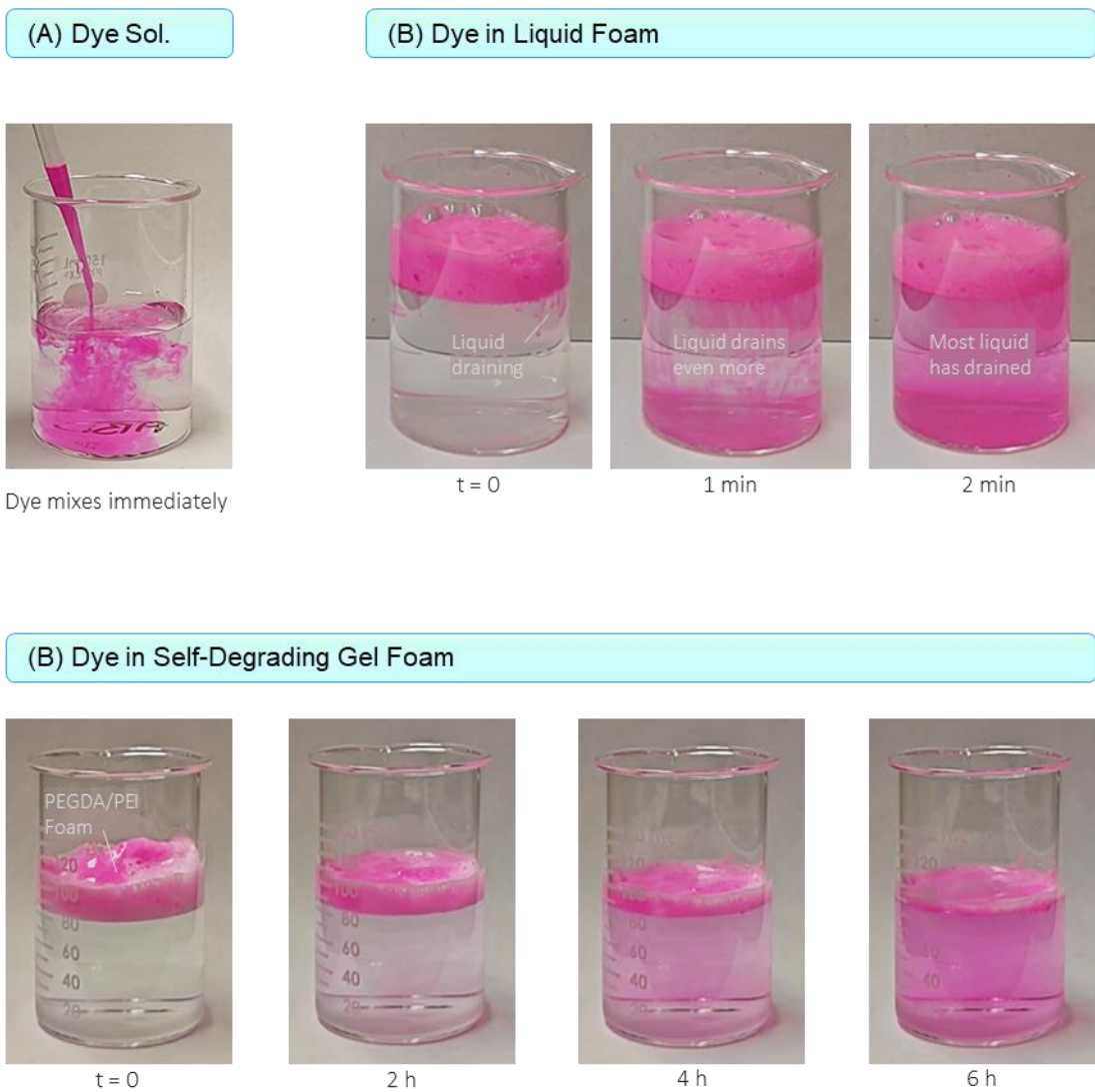
Figure 5.12: Demonstration of controlled release using self-degrading foam. (A) Direct addition of dye solution shows immediate mixing. (B) Conventional liquid foam (2 wt% Tween 80) shows rapid drainage within minutes. (C) Self-degrading gel foam (5 wt% PEGDA/PEI) demonstrates controlled release over 6 hours with eventual complete degradation.
