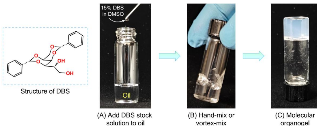
Figure 3.2. DBS organogels and their preparation by a simple new method at room temperature. The structure of DBS is shown in the box. To make the gel, a stock solution of 15% DBS in DMSO is first prepared by simply mixing the two at room temperature. (A) The oil to be gelled is then taken in a vial (here it is 2 g butanol). The stock solution (0.14 g) is added such that the DBS concentration in the mixture becomes 1%. (B) The sample is then mixed by hand or using a vortex mixer for a few seconds. (C) Right afterward, the sample becomes an organogel due to the self-assembly of DBS into a nanofibrillar network. This method to form DBS gels is simple, quick and does not require heat.
