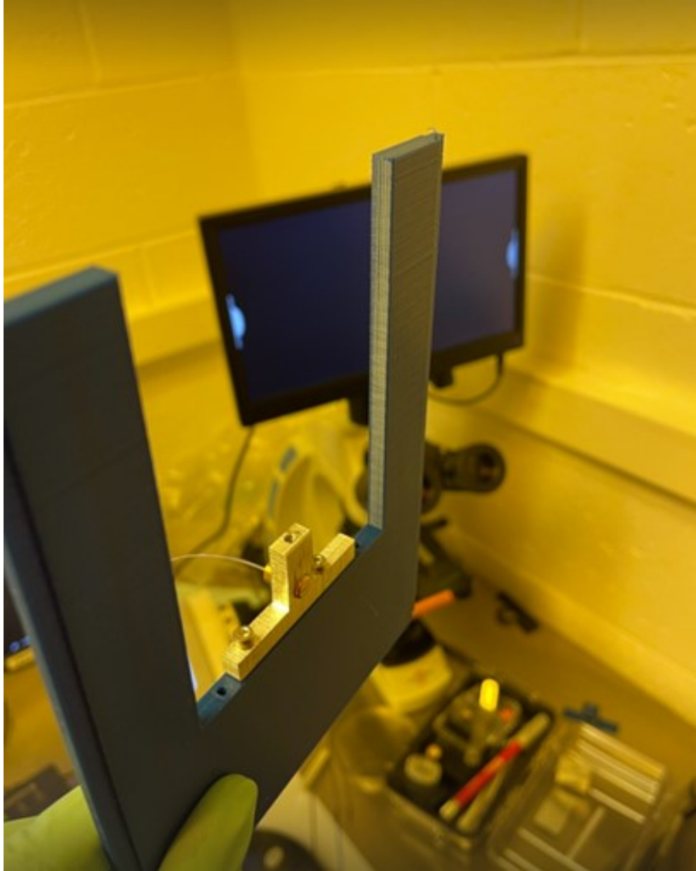
Figure 3.18: Mounting SM fiber: 1st trial- a metal piece was machined with a hole to hold a cut piece of fiber chuck and clamp it from top. This secondary piece is clamped to the primary mount (blue) before putting inside the nanoscribe tool
