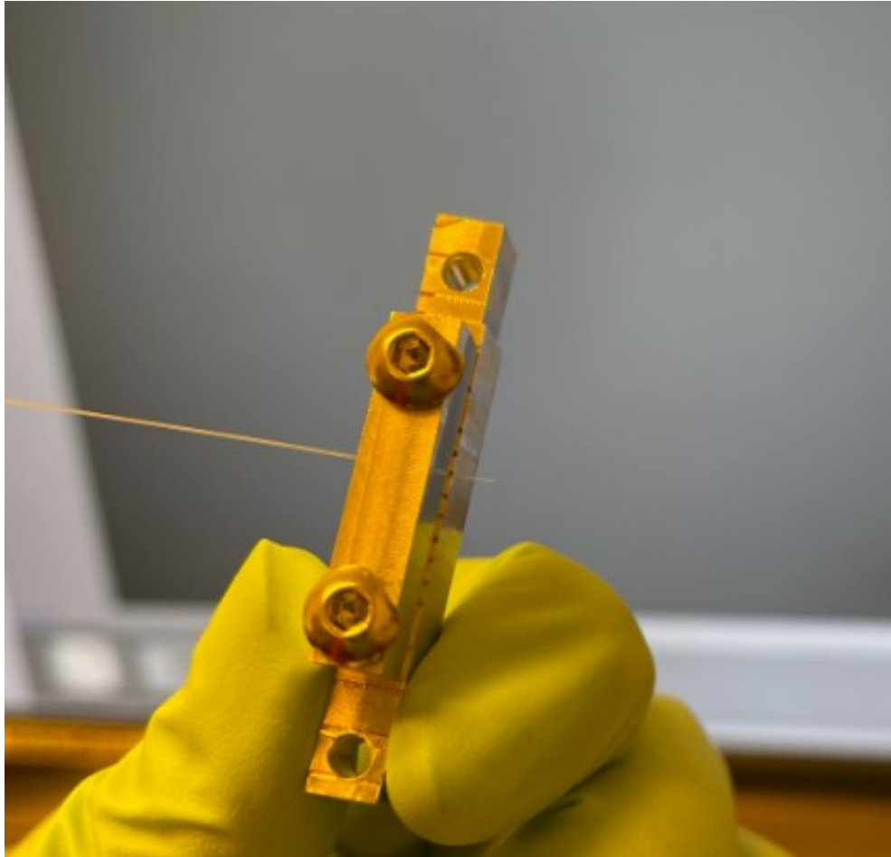
Figure 3.20: Mounting SM fiber: 2nd trial metal piece
