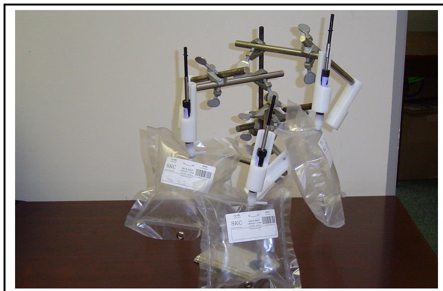
Appendix IV - 6: Exposure of SPME fibers in the Tedlar bag method
