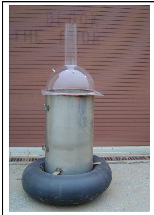
Appendix IV - 2: Designed flux chamber with stack for the secondary aeration tank
