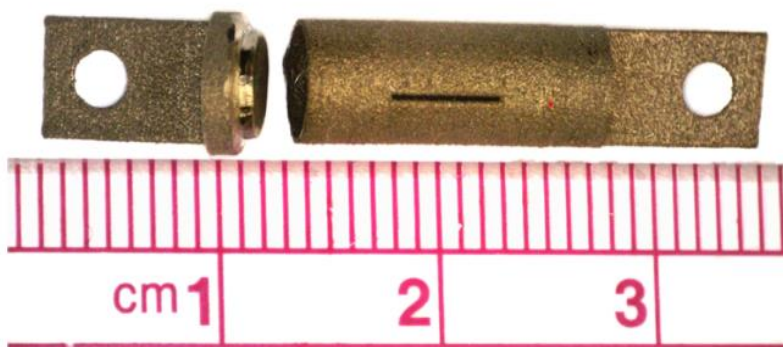
Figure 6-4: 3D printed titanium tube and plug.
