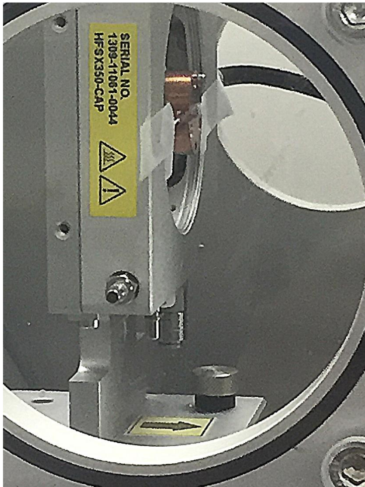
Figure 27. Bundle of UHMWPE fibers mounted on the heating stage for WAXS diffraction.
