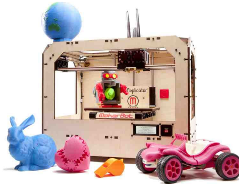
Figure 1: The Makerbot Replicator, a popular, open-source printer, surrounded by printed creations. Strands of solid resin enter the top of the printer, are melted, and are extruded onto the plate (where the completed robot is standing). Image: “The Replicator TM with Prints” by Makerbot Industries on Flickr. Used with a Creative Commons Attribution 2.0 Generic License. http://www.flickr.com/photos/makerbot/6667803681/
