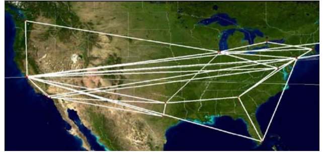
Fig. 2. Exodus US Backbone Topology
