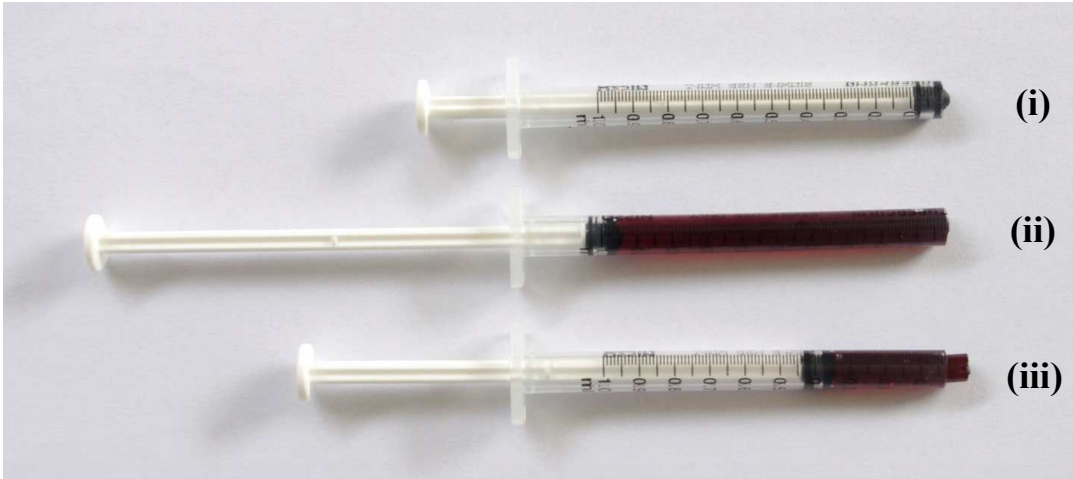
FIGURE E. An empty 1-mL syringe with the tip cut off (i) and a syringe filled with fuchsin glycerin gelatin (ii). The syringe plunger is easily manipulated to control how much gel is used during pollen collection (iii).
