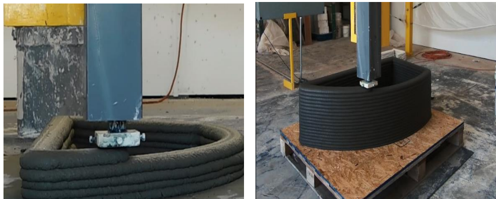
Figure 43. Laticrete’s column printing
