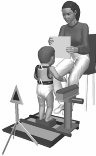
Figure 3.1. An infant stands independently on a pedestal in the no-touch condition. An experimenter sits in front of the infant to keep his/her attention in the task. In the touch condition, the infant's hand lightly touches the bar which is pictured here to the infant's right.
