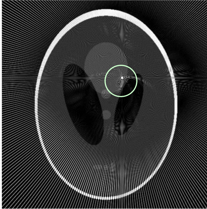
(a) Streak artifacts from the metal after reconstruction using FBP (highlighted for clarity).
