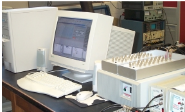
Figure 2.4. Photograph of the dSPACE interface system connected to a PIII-450 MHz PC; setup located in Vibrations Laboratory.
