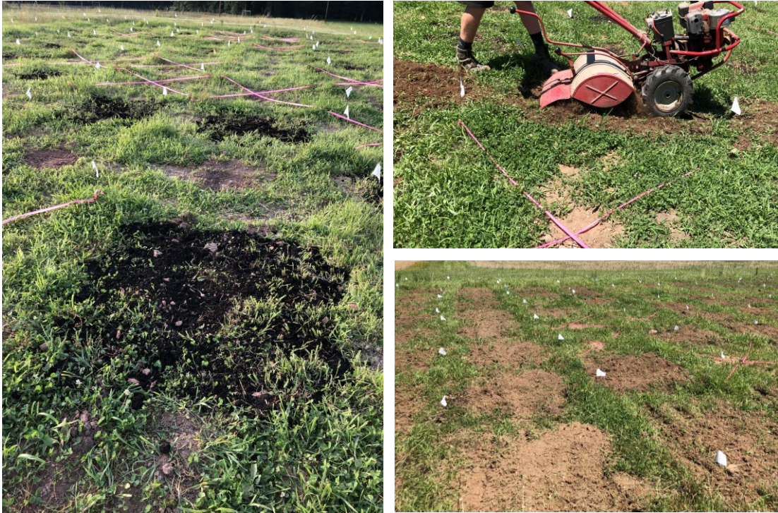
Figure 2.3: (left) Soil amendments top-applied to plots prior to tillage. Untilled control plots are marked with pink tape; (top right) Plots were rototilled following amendment application to a depth of 10cm with a hand-pushed machine rototiller; (bottom right) Treatment plots immediately after tillage at the Beltsville, MD study site.
