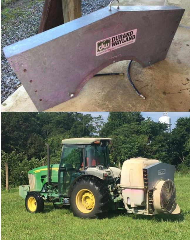
Figure S6. Two-sided row crop head attachment used for 2018 and 2019 airblast sprayer trials detached (top) and mounted to the airblast sprayer (bottom).
