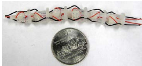
Figure 5: 6-DOF MINIR weighing 2.94 grams
