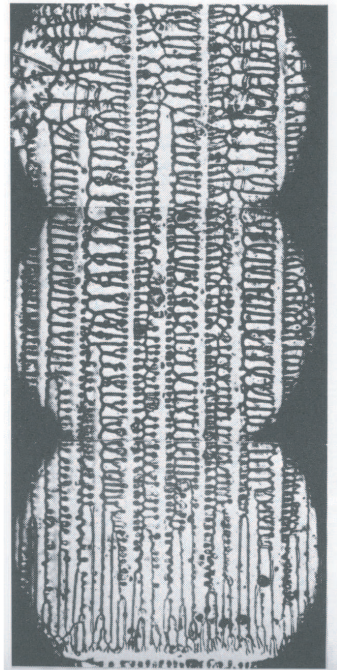
Figure 1.7: A directionally solidified single crystal (tin-1% lead alloy). The black lines indicate the segregation of composition resulted from dendritic growth. (from [1])
