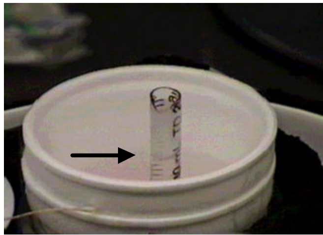
Figure 6.2 A photograph of a liquid nitrogen static pressure test. Arrow indicates liquid column height.
