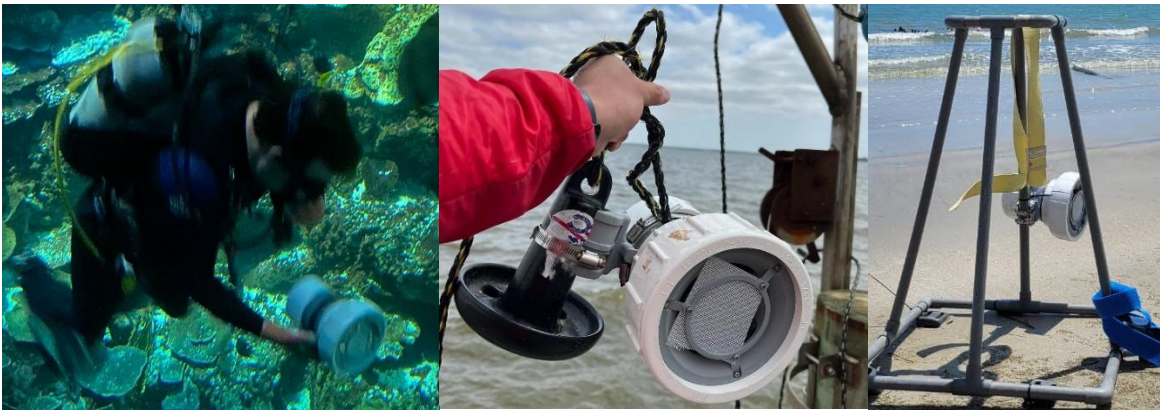
Figure 5: Examples of how the SuMOS can be deployed. Left to right, in calm protected waters with a dive weight, attached to a mushroom anchor off a pier, or on a weighted transect sampler.
