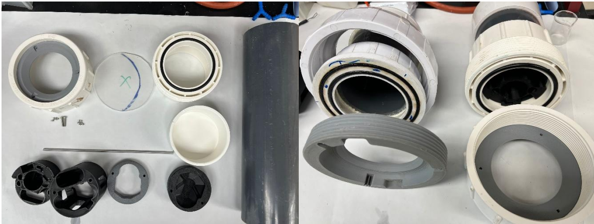
Figure 2: (A, left) Parts for the waterproof enclosure and internal electronic housing, note the O-ring mounting groove on the union fitting. (B, right) Two completed housings using the two configurations of commercially available PVC Unions, as well as substrate mounting flanges. The mounting flange is fitted in the collar of the right one.
