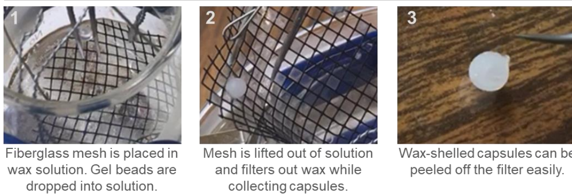
Figure 5.3. Considerations during synthesis of wax-shelled capsules. A) The temperature of the molten (liquid) wax must be above its T_m , but not too high. If the liquid is too hot or if the gel core is incubated in the liquid for too long (> 30 s), the wax shell formed initially will melt and disintegrate. B) Shells can be formed with several waxy materials with varying T_m , as shown in the images (scale bars: 4 mm). For short-chain hydrocarbons like n -eicosane, a second sealing step with octadecane is necessary. C) Several capsules can be coated at once, using a fiberglass mesh to lift out the wax-shelled capsules after incubation.
