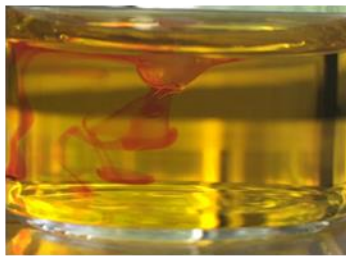
Wax melts, releasing acetic acid
