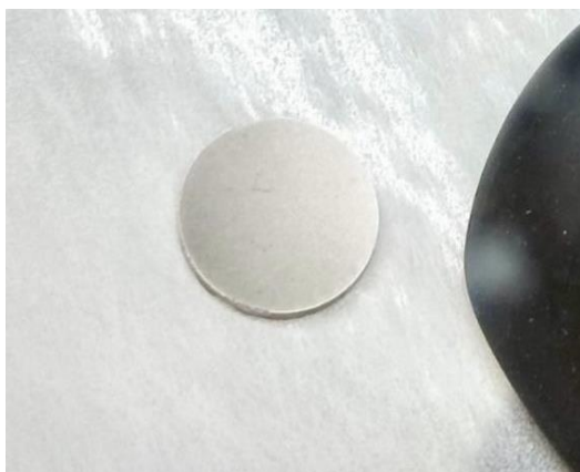
Figure 2.1: \text{Li}_6\text{PS}_5\text{Cl} sulfide solid electrolyte pellet (0.870 mm thick and 0.5 – inch diameter).
