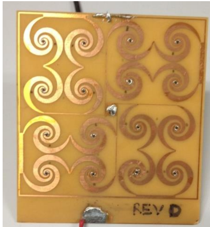
Figure 2.3. The designed broad band rectenna
