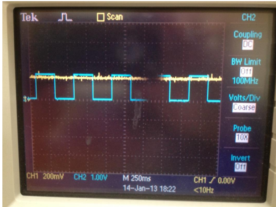
Figure 5.29. Normal operation of the SC voltage converter in the PDS (yellow waveform is the input signal, blue waveform is the output signal)
