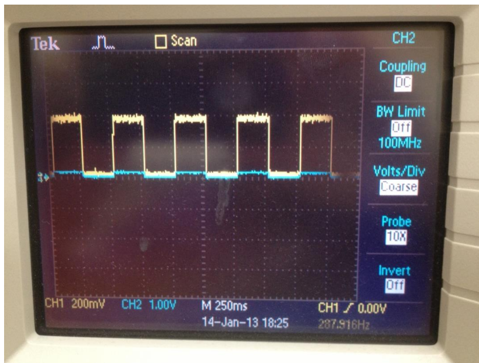
Figure 5.29. Normal operation of the SC voltage converter in the PDS (yellow waveform is the input signal, blue waveform is the output signal)
