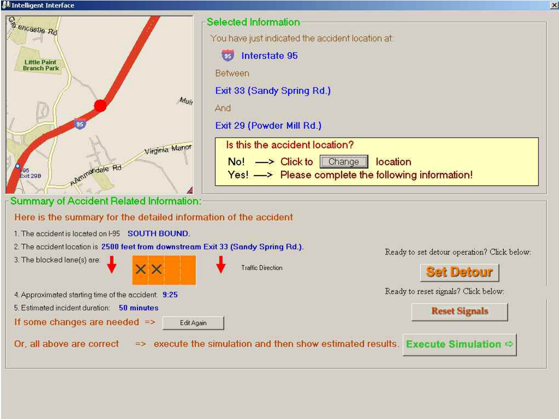
Figure 6-10 A summary screen for users to review all input information for simulating incident impacts
