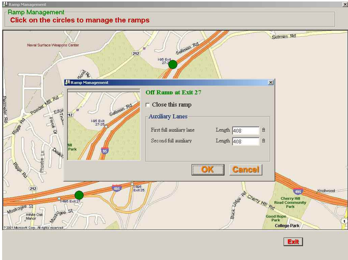
Figure 6-13 The interface for users to close the ramp and/or change the length of the auxiliary lanes
