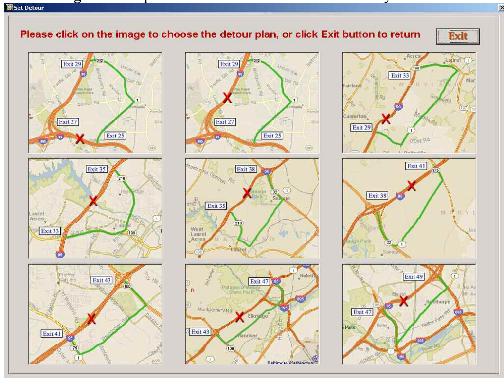
Figure 4-4 9 preset detour routes for I-95/Route-1 by MDSHA
