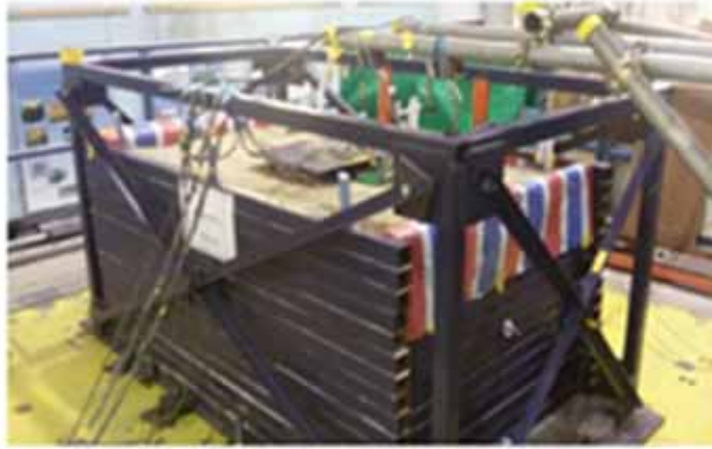
Figure 4-8: The physical model used for shaking table tests (after Komak Panah et al. 2018)
