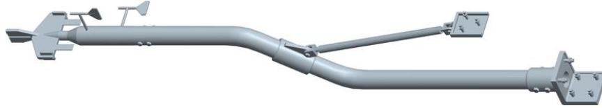
Figure 4.7: Unsimplified boom model for a modal analysis
