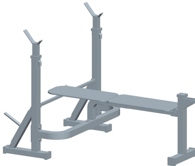
Figure 4.13: Unsimplified weight bench assembly model for a structural analysis
