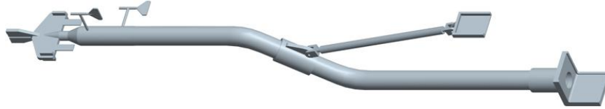
Figure 4.8: Simplified boom model for a modal analysis
