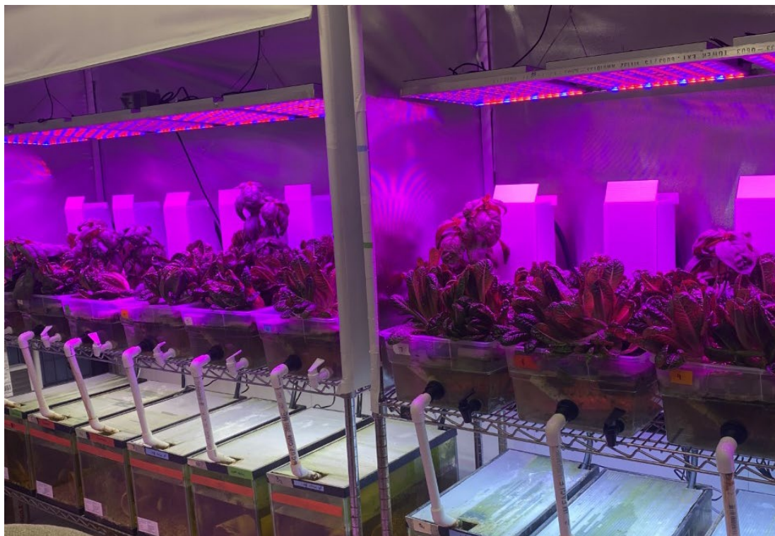
Figure 3. 1 setup of recirculating research aquaponics systems and discharge tube connecting grow bed to fish tank. Mature lettuce and basil are shown in the raft.
