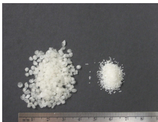
Figure 5.2: Relative size of capsules prepared by using a syringe and a nozzle.
