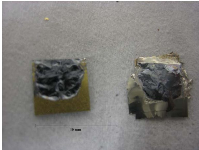
Figure 17: Partially wetted die and solder layers
