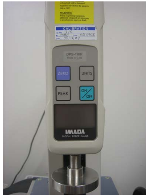
Figure 14: Digital force gauge (110 lb maximum 0.1 lb resolution)
