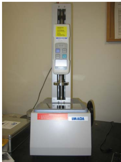
Figure 13: IMADA manual load cell used to apply pressure to samples
