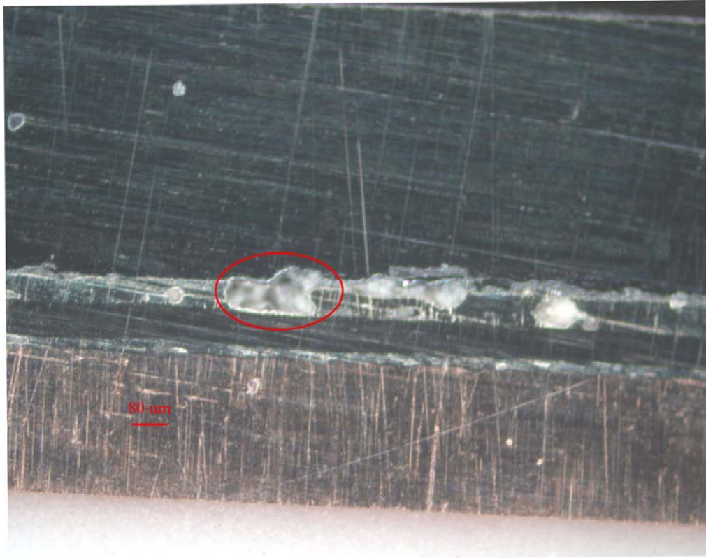
Figure 31: Voiding within completed samples
