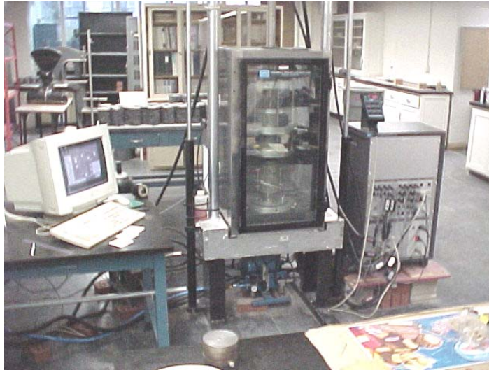
Figure 12. UTM-100 testing system.
