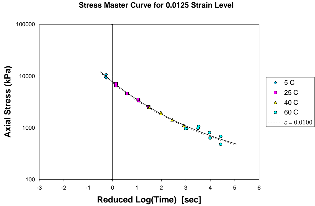
Figure 58. Stress vs. reduced time master curve for 0.0125 \epsilon from strain rate tests.
