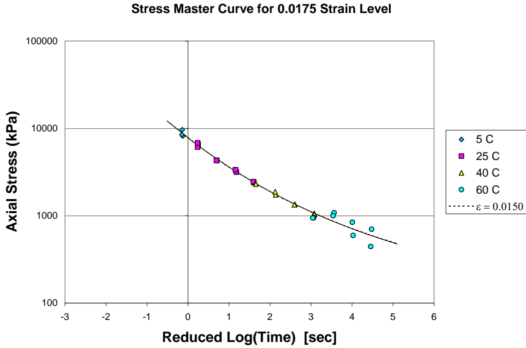
Figure 60. Stress vs. reduced time master curve for 0.0175\epsilon from strain rate tests.
