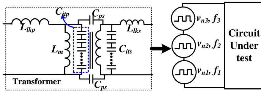
Fig. 5. 3. Equivalent noise model of PSFB converter
