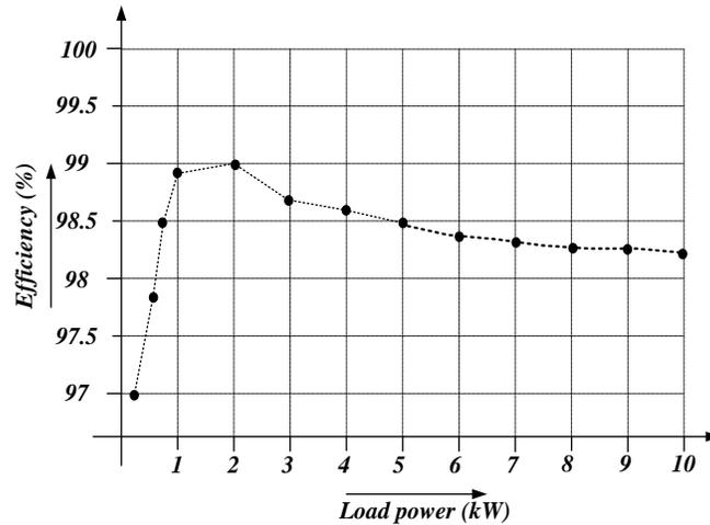
Fig. 2.14. (a) Efficiency of the three-phase boost PFC versus output power (kW).
