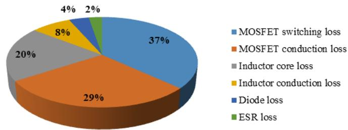
Fig. 2.14. (b) Power loss split in different components.
