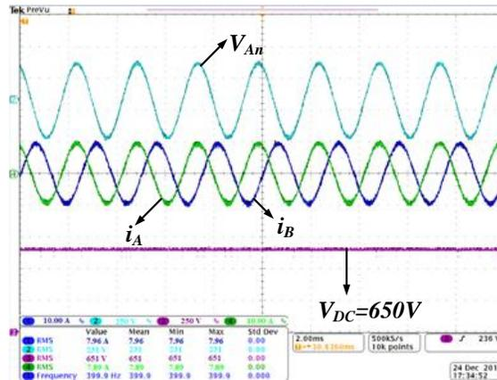
Fig. 3.11. 6kW PFC waveforms at 400Hz with the proposed control
