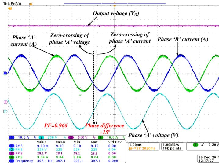
Fig. 6. 9. PFC stage waveforms @ 6kW, 230V AC input
