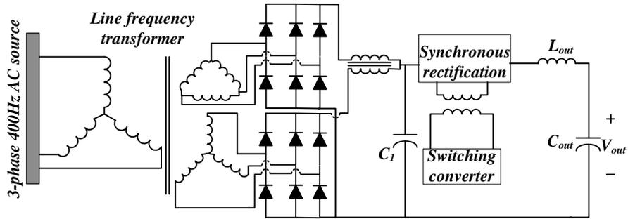
Fig. 1.3(b) Transformer rectifier unit structure proposed in [6]
