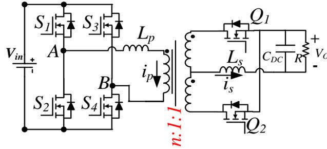
Fig. 4. 1. Basic structure of a center-tapped PSFB DC-DC converter.
