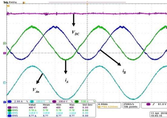
Fig. 2.23. Experimental waveforms of the converter; phase currents:  $i_A$  (RMS) =  $i_B$  (RMS) = 6.18A
