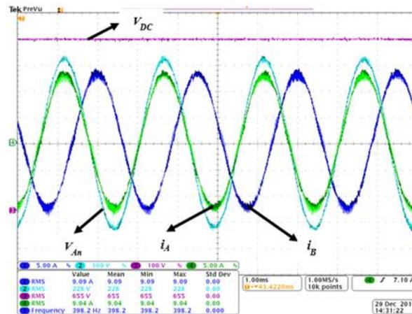
Fig. 6. 10.  $V_{DC}=650V$ ,  $i_A$  (RMS) =  $i_B$  (RMS) = 9.06A,  $V_{An}$  (RMS) = 230V @ 6kW
