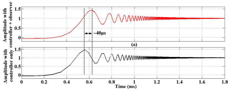
Fig. 6. 6. Closed loop step-response of phase ‘B’ current with and without observer at poles (repeated - 50kHz)
