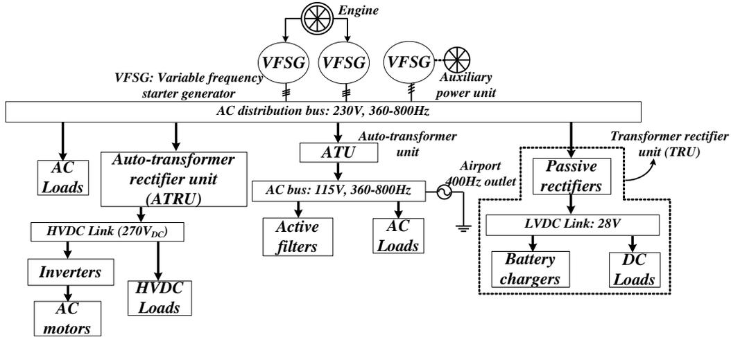
Fig. 1.4. Electrical power system architecture inside Boeing 787 Dreamliner [12]
