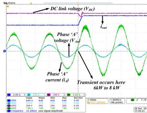
Fig. 3.15. PFC waveforms under load transient (6 kW to 8kW) with the proposed integrated control
