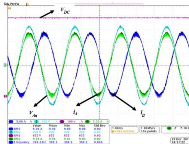
(a)  $V_{DC}=650V$ ,  $i_A$  (RMS) =  $i_B$  (RMS) =  $9.06A$ ,  $V_{An}$  (RMS) =  $230V$ ,  $P_{out}=6kW$
