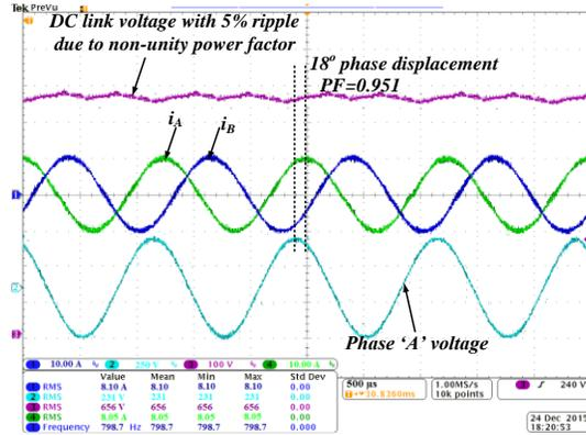
Fig. 3.12. 6kW PFC waveforms at 800Hz with the conventional control
