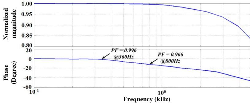
Fig. 3.4. Bode plot of the closed loop transfer function with PI compensator
