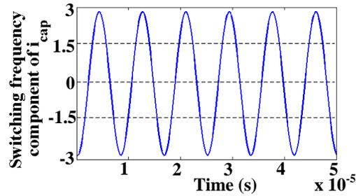
Fig. 7.5. Switching harmonic of capacitor ripple current
