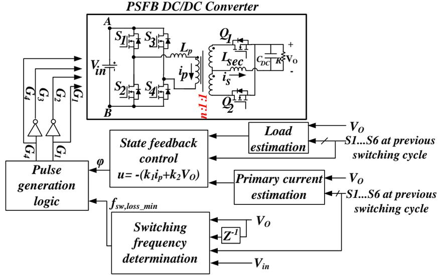
Fig. 4.4. Variable switching frequency state-feedback controller of PSFB converter.
