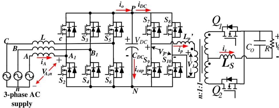
Fig. 7.1. Structure of the integrated three-phase boost PFC and PSFB converter.
