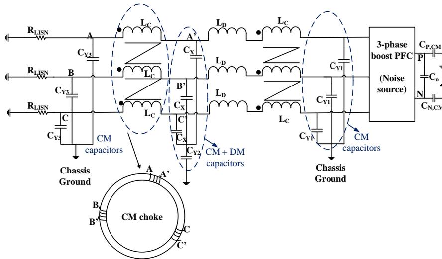
Fig. 5. 6. Cascaded two-staged EMI filter for three-phase boost PFC
