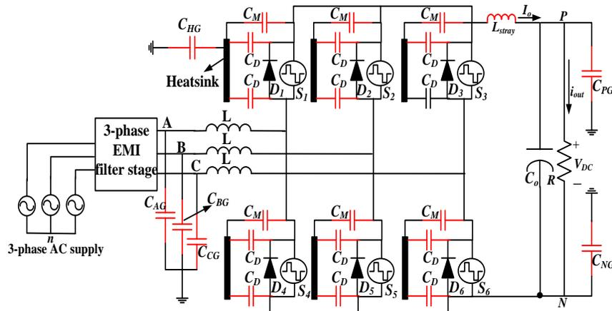
Fig. 5. 2. Noise modeling in a three-phase boost PFC converter.
