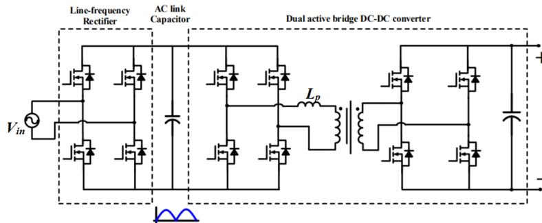
Fig. 8.5. Indirect matrix-based single-stage AC-DC converter topology(alternative-4)
