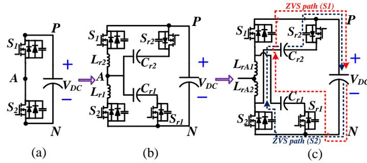
Fig. 2.17. (a) One phase-leg (b) one phase-leg with ZVS circuit (c) one phase-leg with modified soft-switching circuit
