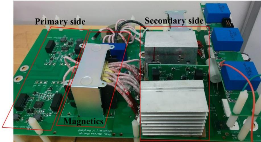
Fig. 4.9. Photo of the PSFB DC-DC experimental setup
