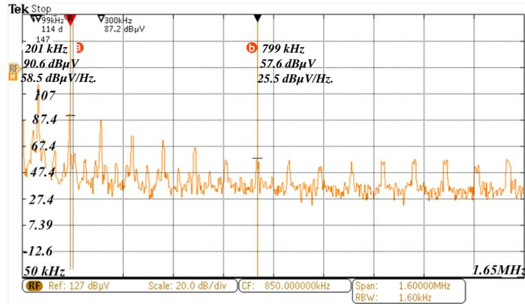
Fig. 5. 4. DM zone EMI results of PFC stage without any filter
