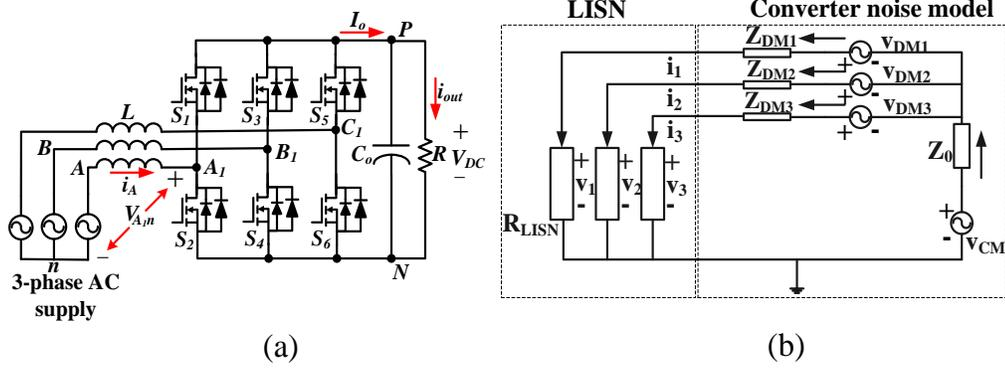
Fig. 5.1. (a) Three-phase boost PFC (b) High-frequency noise model of a three-phase PWM rectifier with LISN.
