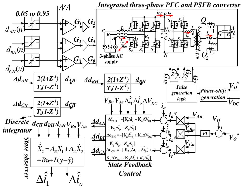
Fig. 6. 4. Control Strategy of the integrated PFC and PSFB converter
