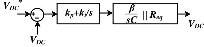
Fig. 7.10. Voltage control loop for three-phase PFC
