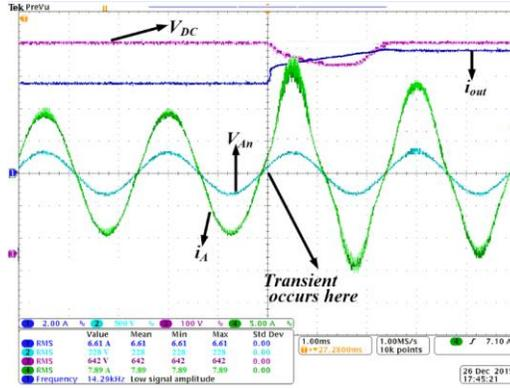
Fig. 3.14. PFC waveforms under load transient (6 kW to 8kW) with PI control
