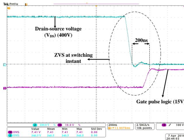
Fig. 2.24. ZVS of a main switch: drain-source voltage of  $S_1$ , gate pulse of  $S_1$
