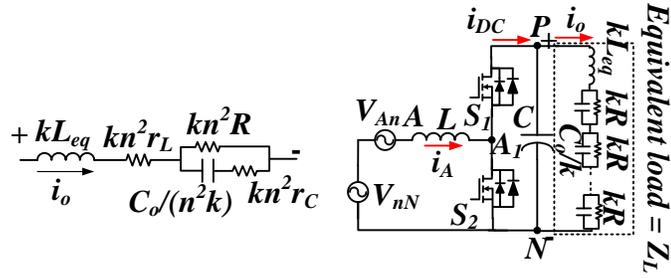
Fig. 6. 2. (a)The DC-DC converter model as an equivalent load to the PFC (b) One phase of the integrated converter
