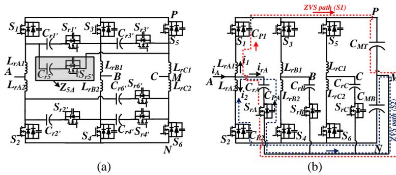
Fig. 2.19. (a) Second modified soft-switched three-phase PFC legs (b) Third modified soft-switched three-phase legs with reduced number of capacitors
