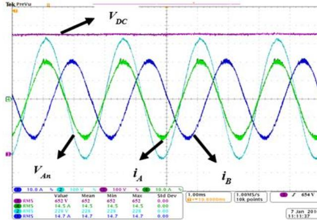
(a)  $V_{DC}=652V$ ,  $i_A$  (RMS) =  $i_B$  (RMS) = 14.6A,  $V_{An}$  (RMS) = 230V,  $P_{out}=9.8kW$
