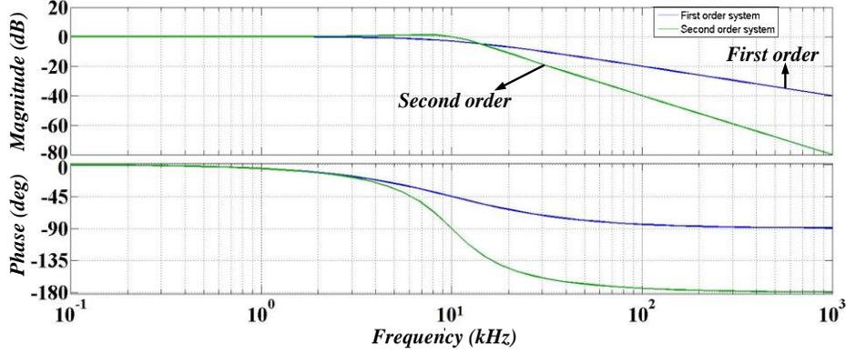
Fig. 3.7. First and second order systems with corner frequency of 10 kHz.
