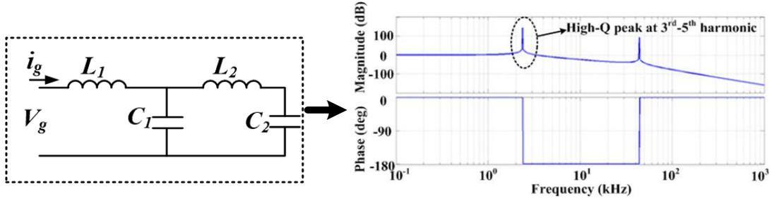
Fig. 5. 9. Frequency response of a two-stage LC filter without damping
