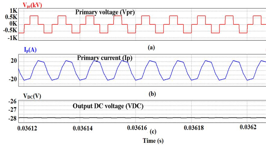
Fig. 4.8. Simulation results of PSFB converter (a) Primary voltage ( $V_{pr}$ ) (b) Primary current ( $i_{pr}$ ) (c) Output DC voltage ( $V_{DC}$ )
