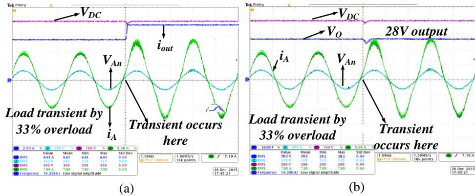
Fig. 7.16. The converter waveforms under load transient from 6kW to 8kW.
