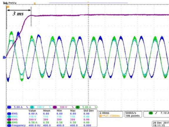
Fig. 3.10. PFC converter waveforms during start-up action with the proposed integrated control
