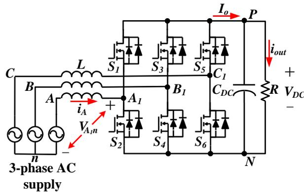
Fig. 2.1 Three-phase boost PFC rectifier
