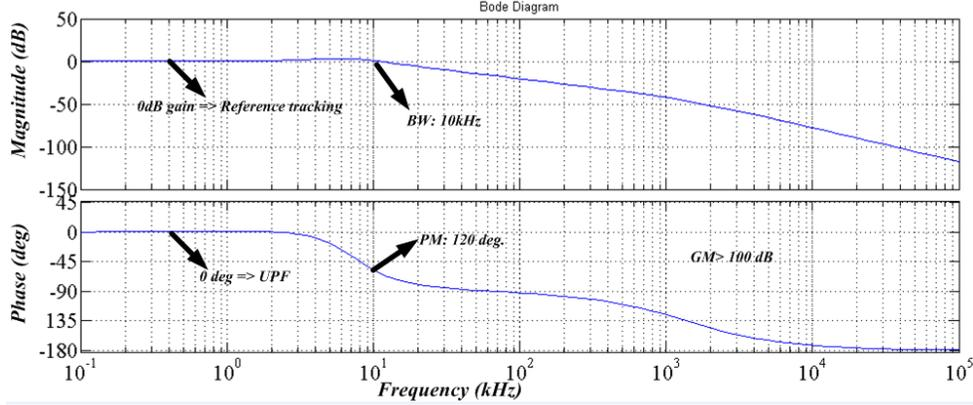
Fig. 5. 11. Frequency response of a two-stage LC filter with damping
