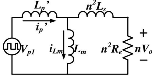
Fig. 4.3. Reduced equivalent circuit from FHA of PSFB converter.
