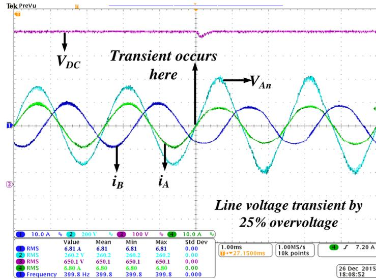
Fig. 2.12. Experimental waveforms of the converter under input line transient from 230V to 285V phase-neutral RMS at 400Hz source frequency and  $V_{DC}=650V$ .
