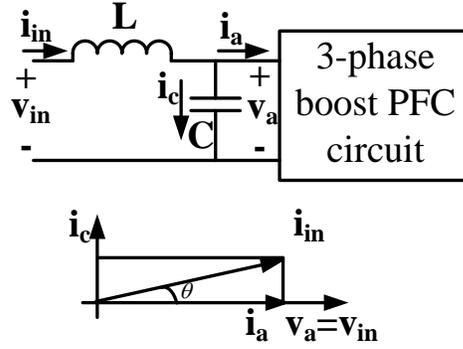
Fig. 5. 5. Phasor diagram of a single-stage LC filter before PFC circuit.
