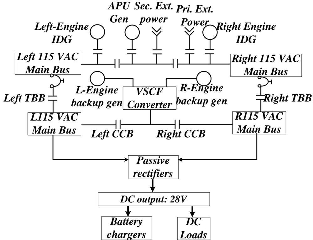
Fig.1.1. Electrical power generation and distribution architecture inside Boeing 777
