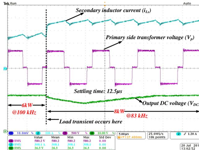
Fig. 4.13. PSFB waveforms at load transient from 6kW to 8kW in variable switching frequency, PI control;  $V_{in} = 650V$ ,  $V_O = 28V$ ,  $f_{sw} = 100\text{kHz}$  @6kW and  $f_{sw} = 83\text{kHz}$  @8kW.
