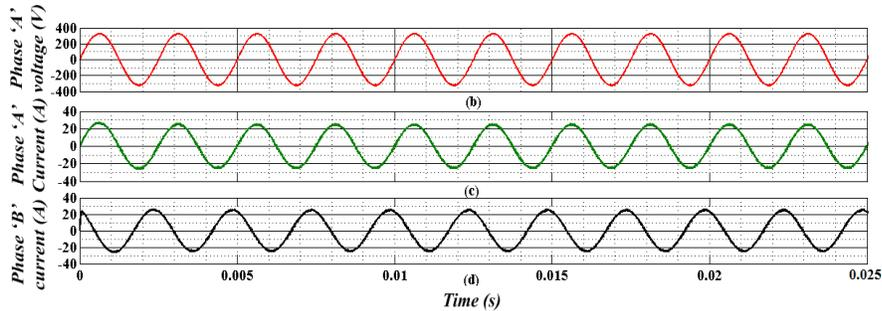
Fig. 2.6. Simulation results of three-phase boost PFC at 10kW power with the proposed control (with injection of common-mode duty ratio).
