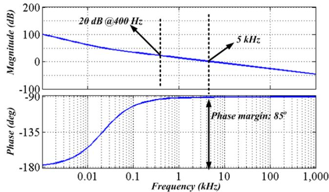
Fig. 7.8. Open loop Bode plot of the proposed control loop
