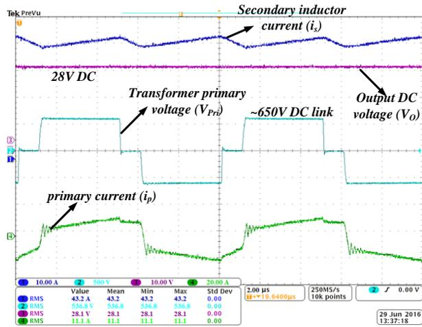
Fig. 6. 23. 6kW PSFB stage waveforms
