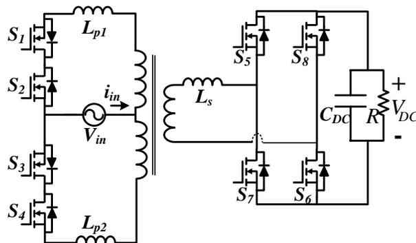
Fig. 8.6. Single-stage AC-DC converter in push-pull configuration (alternative-5)
