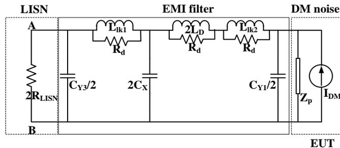
Fig. 5. 10. A two-stage LC filter with damping
