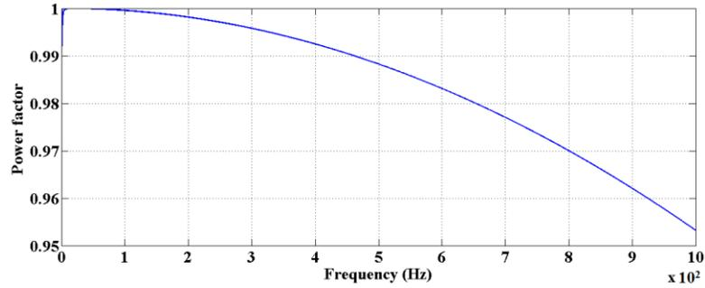
Fig. 3.6. Variation of power factor with source frequency
