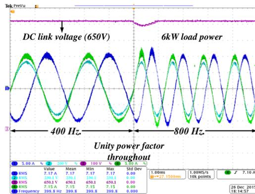
Fig. 3.13. Unity power factor at two extremum frequencies in the six-switch PFC at 6kW
