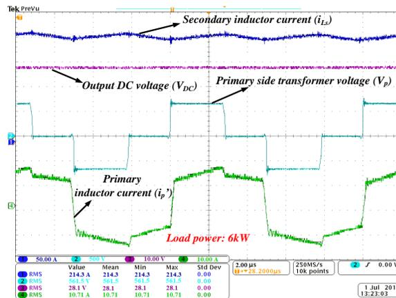
Fig. 7.13. PSFB waveforms at 6kW load power;  $V_{DC} = 650V$ ,  $V_O = 28V$ .
