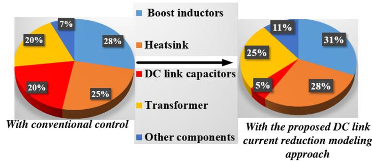
Fig. 7.19. The weight split of components in the cascaded AC-DC stage.
