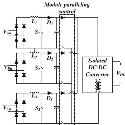
Fig. 1.3(c) Transformer rectifier unit structure proposed in [7]
