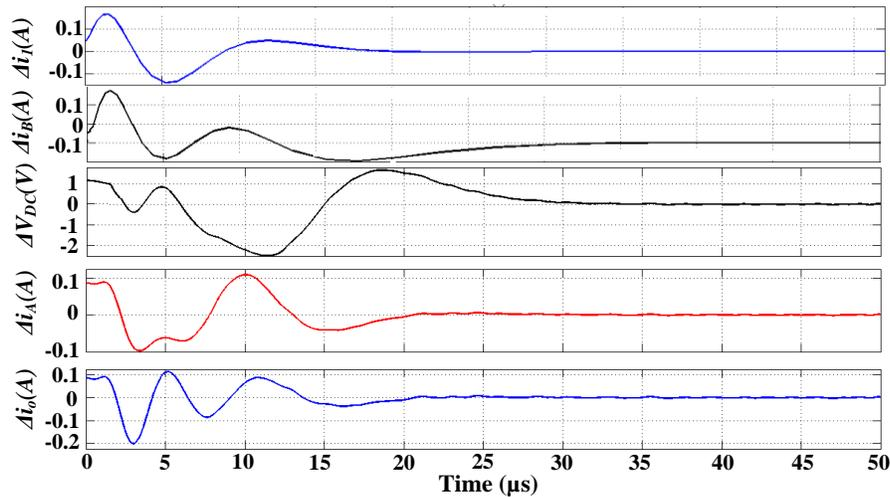
Fig. 6. 8. Changes in State variables under 10MHz Gaussian disturbance
