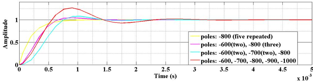
Fig. 6. 5. Step response of  $V_{DC}(s)/V_{DC}^*(s)$  at different pole locations
