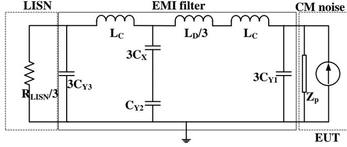
Fig. 5. 7. CM equivalent of the proposed EMI filter for three-phase boost PFC
