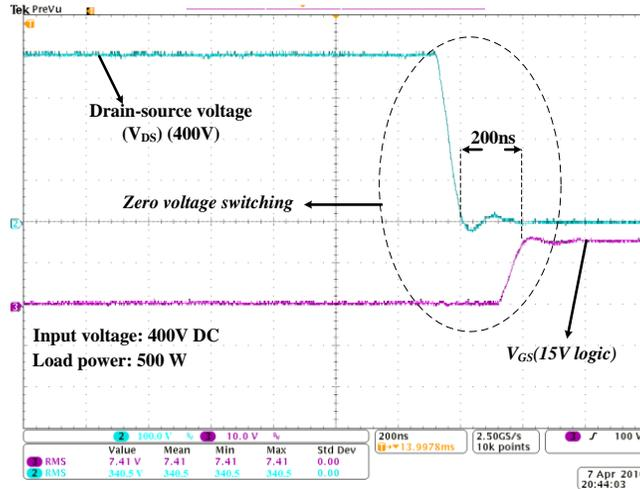
Fig. 4.11. ZVS in PSFB converter at 500W load power  $V_{in} = 400V$ ,  $V_O = 20V$ , Output current: 25A.
