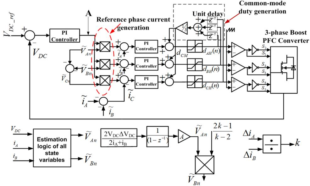
Fig. 2.2. Block diagram of the proposed control system for a three-phase active boost rectifier
