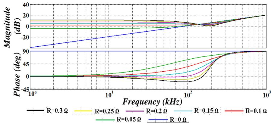
Fig. 4.5. Bode plot of the input impedance of PSFB converter.
