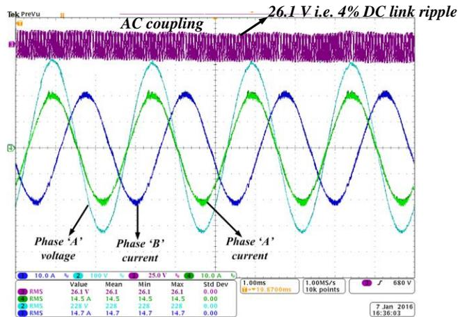
Fig. 7.14. Voltage and current waveforms of the 6kW three-phase inverter experiment with conventional control: 4% DC voltage ripple with 45 $\mu$ F capacitance (as seen from the AC coupling measurement of DC link voltage)
