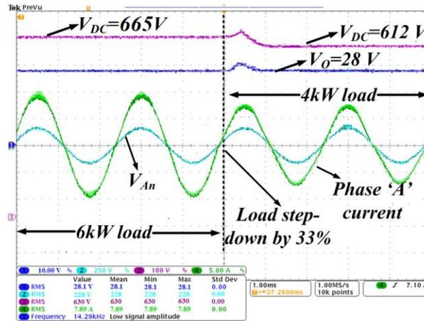
Fig. 6. 24. A load transient from 6kW to 4kW in the integrated RTRU, demonstrating the change in intermediate DC link voltage from 665V to 612V
