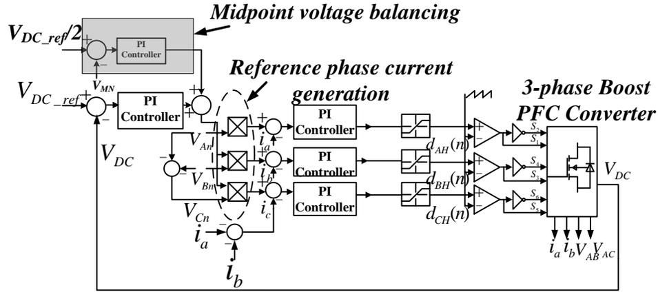
Fig. 2.22. DC link midpoint voltage balancing logic of a three-phase PFC
