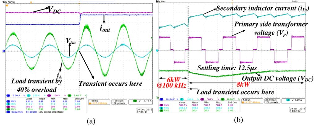
Fig. 6. 12. (a) The converter waveforms under load transient from 6kW to 8kW (b) PSFB waveforms at load transient from 6kW to 8kW;  $V_{DC} = 650V$ ,  $V_O = 28V$ ,  $f_{sw} = 100$  kHz.
