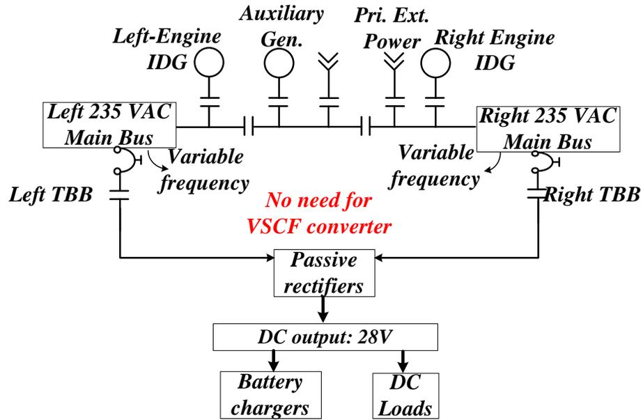
Fig. 1.2. Electrical power generation and distribution architecture inside Boeing 787
