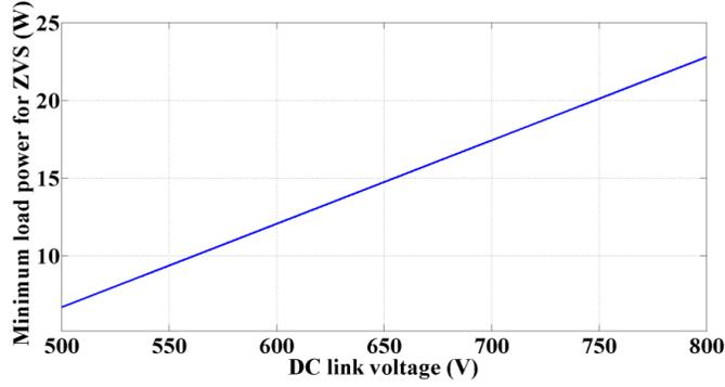
Fig. 6. 18. Minimum load power for ZVS with varying DC link voltage
