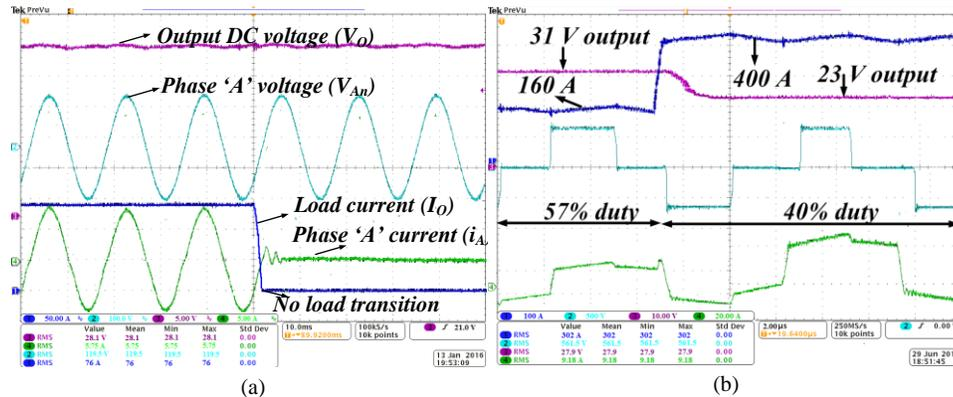
Fig. 6. 14. (a) Converter waveforms at no-load condition (b) PSFB stage waveforms during short circuit test
