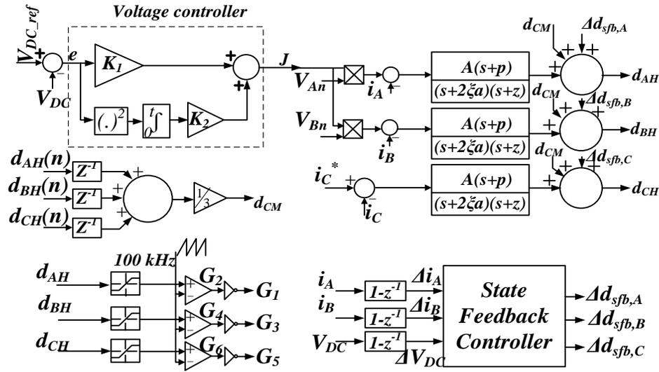
Fig. 3.3. The proposed control block diagram
