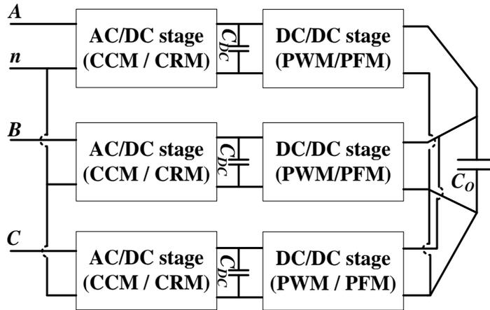
Fig. 8. 7. Two-stage modular RTRU with neutral access requirement (alternative-6)
