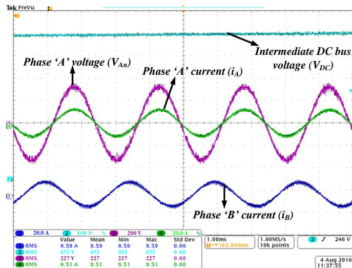
Fig. 6. 22. 6kW PFC stage waveforms (at 230V 400Hz AC input)
