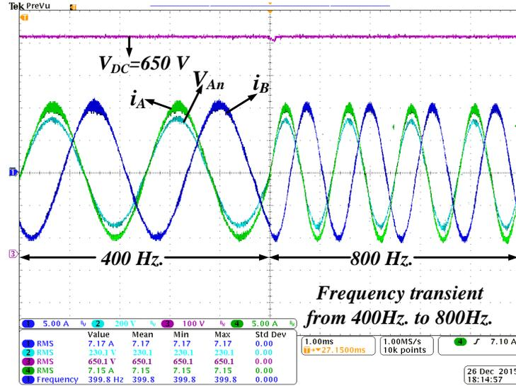
Fig. 2.13. Experimental waveforms of the converter under input frequency transient from 400Hz to 800 Hz at 230V phase-neutral RMS and  $V_{DC}=650V$ .
