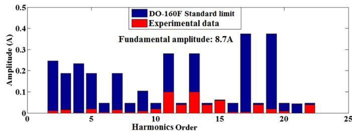
Fig. 7.18. FFT amplitudes of lower order grid frequency harmonics (800 Hz (2<sup>nd</sup> harmonic) to ~9kHz (22<sup>nd</sup> harmonic))
