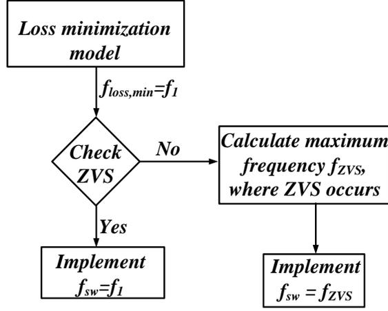
Fig. 4.7. Flowchart for the switching frequency selection procedure.
