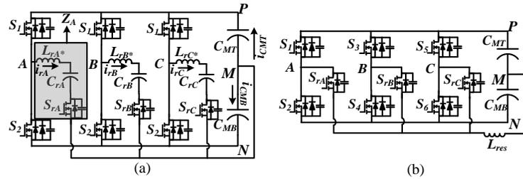
Fig. 2.20. (a) Fourth modified soft-switched three-phase legs (b) Final proposed soft-switched structure of three-phase legs
