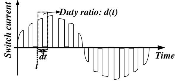
Fig. 6.15. Typical PFC switch current waveform
