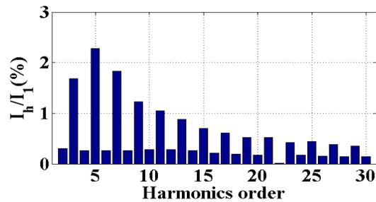
Fig. 5. 15. Harmonic spectrum of phase current at rated input and 10kW load.
