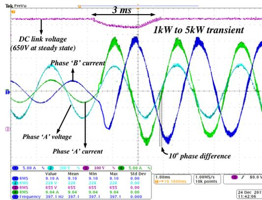
Fig. 3.18. Load transient of PFC converter from 1kW to 5kW using PI compensation
