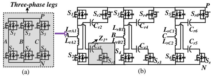
Fig. 2.18. (a) Three-phase legs (b) Three-phase legs with first modified soft-switching auxiliary circuit
