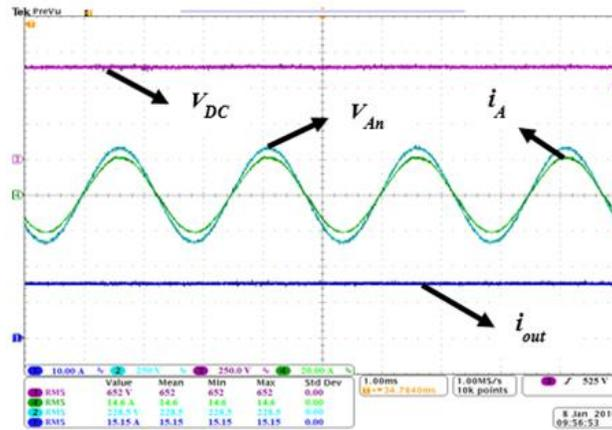
(b)  $V_{DC}=650V$ ,  $i_{out}=15.15A$ ,  $i_A$ (RMS)=14.6A,  $V_{An}$ (RMS)=230V,  $P_{out}=9.8kW$
