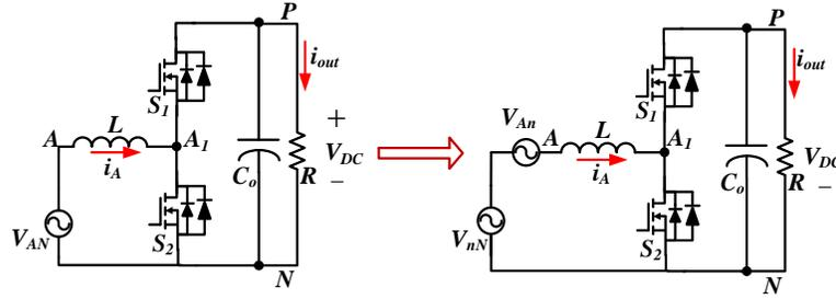
Fig. 2.3. One independent leg of a three-phase active boost-type rectifier.
