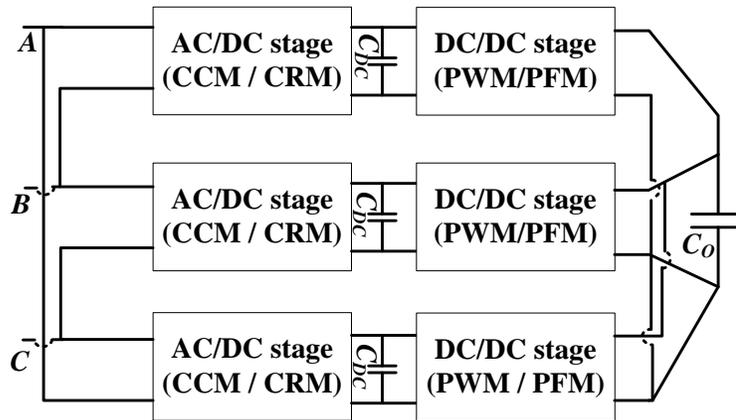
Fig. 8. 8. Two-stage modular RTRU with no neutral access requirement (alternative-7)
