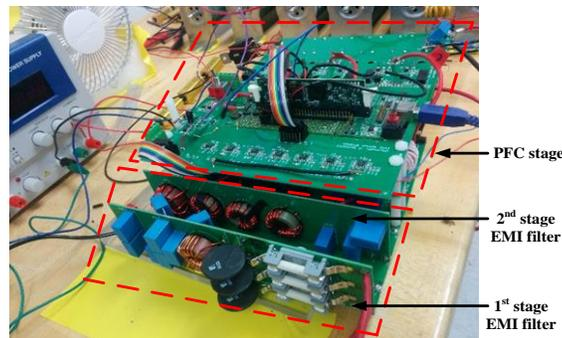
Fig. 5. 12. Photo of the integrated EMI and three-phase boost PFC prototype.
