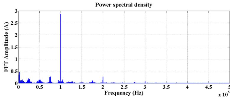
Fig. 7.6. FFT of the DC link capacitor current ( $i_{cap}$ )
