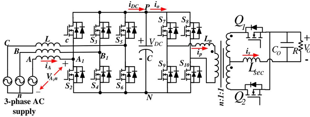
Fig. 6. 1. Integrated two stage AC-DC converter for RTRU
