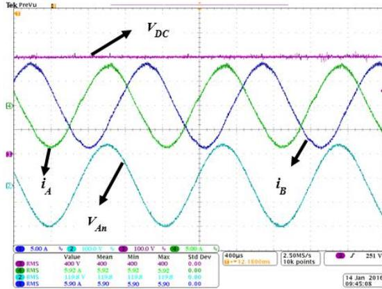
Fig. 2.11. Experimental waveforms of the converter at 800Hz source frequency & 2.1kW load power
