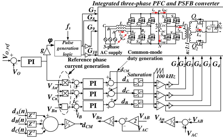
Fig. 7.2. The control block diagram without DC link current minimization logic
