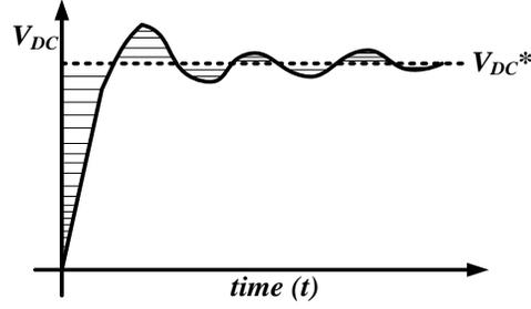
Fig. 3.2. A typical waveform for the DC link voltage settling
