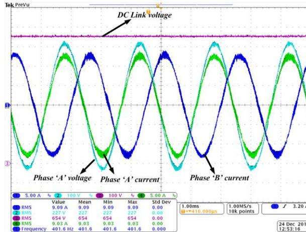
Fig. 7.12.  $V_{DC}=650V$ ,  $i_A=i_B=9.06A$  (RMS),  $V_{An}$  (RMS) =230V,  $P_{out}=6kW$ .
