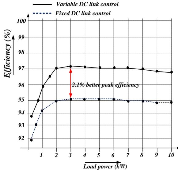
Fig. 6.25. Efficiency comparison between fixed DC link and variable DC link control
