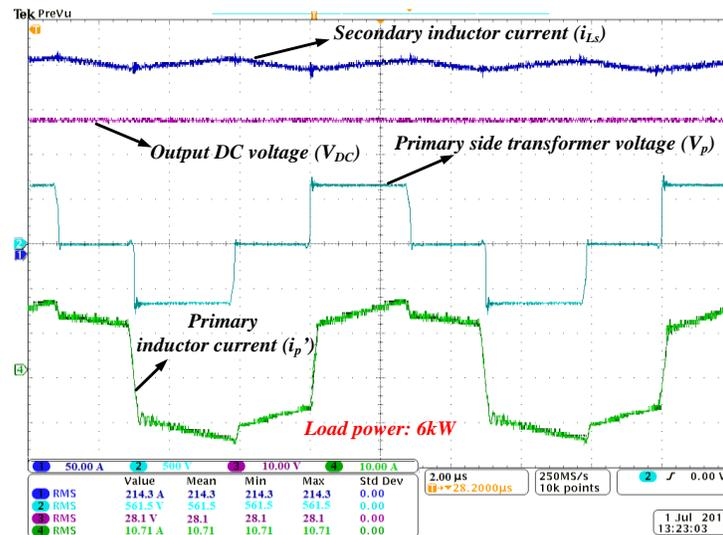
Fig. 4.10. PSFB waveforms at 6kW load power;  $V_{in} = 650V$ ,  $V_O = 28V$ , Output current: 214.3A.
