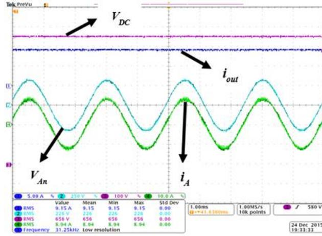
(b)  $V_{DC}=650V$ ,  $i_{out}=9.15A$ ,  $i_A$  (RMS) =9A,  $V_{An}$  (RMS) =230V,  $P_{out}=6kW$
