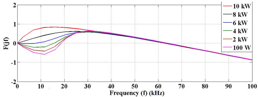
Fig. 4.6. Variation of cut-in frequency of ZVS occurrence in PSFB converter.
