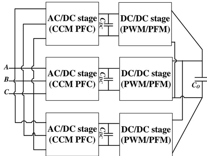
Fig. 8. 1. 3-phase modular RTRU (alternative-1)
