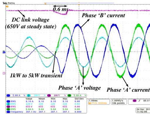
Fig. 3.17. Load transient of PFC converter from 1kW to 5kW using the proposed control
