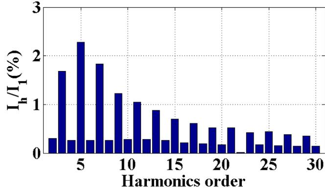
Fig. 2.15. Harmonic spectrum of phase current at rated input and 10kW load power
