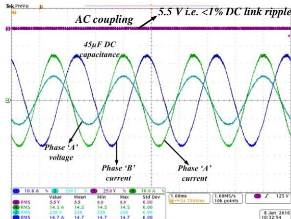
Fig. 7.15. Voltage and current waveforms of the 6kW three-phase inverter experiment with the proposed control: 1% DC voltage ripple with 45 $\mu$ F capacitance (as seen from the AC coupling measurement of DC link voltage).
