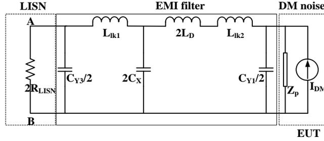
Fig. 5. 8. DM equivalent of the proposed EMI filter for three-phase boost PFC
