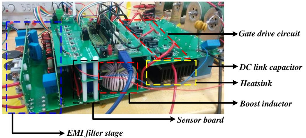
Fig. 2.8. Photo of the three-phase boost PFC prototype.
