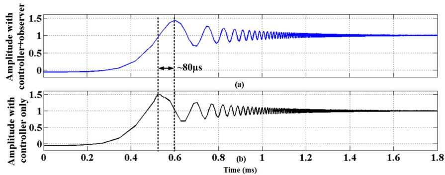
Fig. 6. 7. Closed loop step-response of phase ‘B’ current with and without observer at poles (two at - 50kHz, one at -30kHz)
