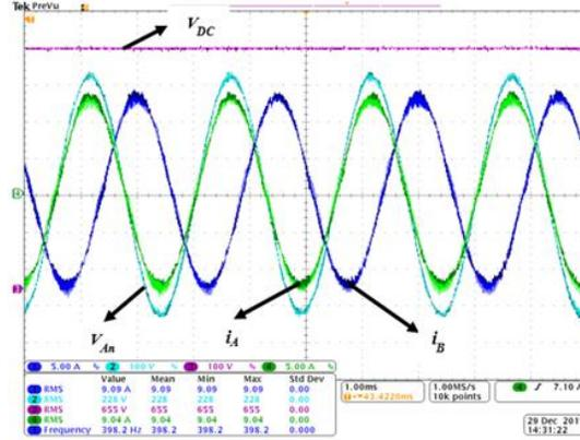
Fig. 5. 14. Experimental waveforms of the converter at 6kW (a) Phase ‘A’ voltage and current, Phase ‘B’ current, DC link voltage.  $V_{DC}=650V$ ,  $i_A$  (RMS) =  $i_B$  (RMS) =  $9.06A$ ,  $V_{An}$  (RMS) =  $230V$ ,  $P_{out}=6kW$ .
