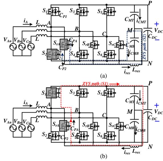
Fig. 2.21. Final proposed soft-switched 3-phase boost PFC structure (a) ZVS path of  $S_2$  in the finally proposed soft-switched structure of three-phase PFC (b) ZVS path of  $S_1$  in the proposed soft-switched PFC structure
