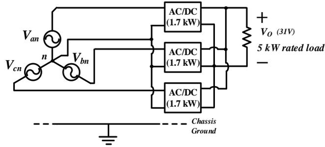
Fig. 8. 3. The proposed converter topology in a 3-phase 5-wire system
