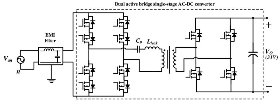
Fig. 8. 4. Schematic showing the converter topology along with the EMI filter (alternative-3)
