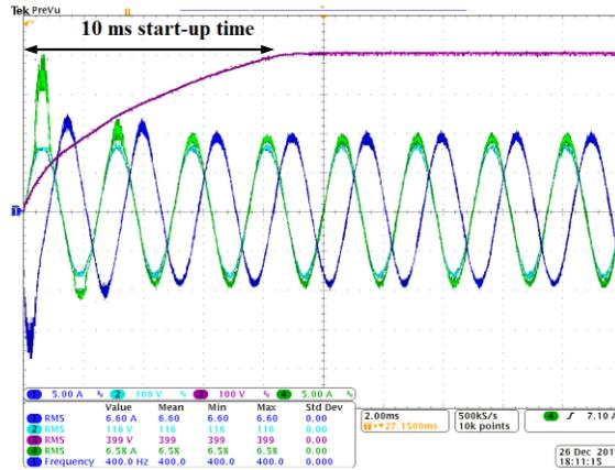
Fig. 3.9. PFC converter waveforms during start-up action with PI compensation
