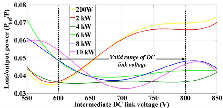
Fig. 6. 20. Total power loss variation with intermediate DC voltage levels a different load power
