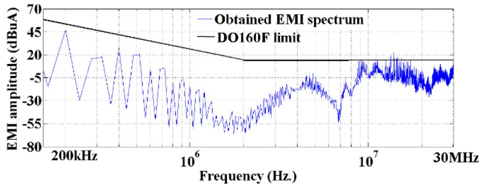
Fig. 5. 13. EMI spectrums over entire conducted EMI range after applying the proposed EMI filter.
