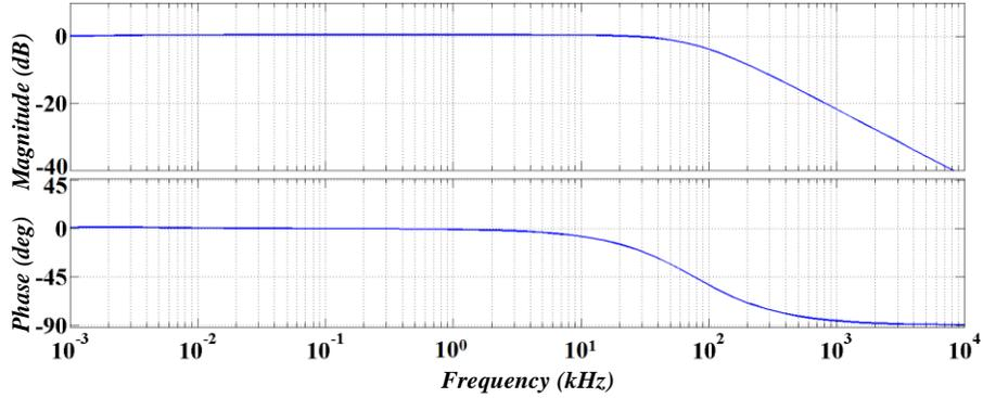
Fig. 3.8. Bode plot of the closed loop system with the proposed controller
