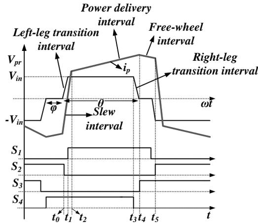
Fig. 4.2. Typical waveforms of primary voltage, primary current and gate pulses in a PSFB converter. During ZVS phase-shift operation of the converter, there are five states in a half-cycle of operation. These states are briefly discussed due to the symmetric operation of the circuit.
