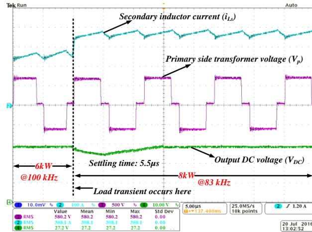
Fig. 4.12. PSFB waveforms at load transient from 6kW to 8kW in variable switching frequency, state-feedback control;  $V_{in} = 650V$ ,  $V_O = 28V$ ,  $f_{sw} = 100\text{ kHz}$  @6kW and  $f_{sw} = 83\text{kHz}$  @8kW.
