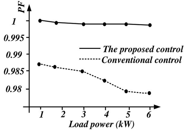
Fig. 6. 3. Power factor variation over load power at two different control strategies
