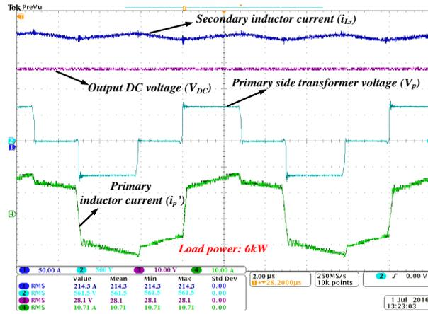
Fig. 6. 11. PSFB waveforms at 6kW load power;  $V_{DC} = 650V$ ,  $V_O = 28V$ , Output current: 214.3A
