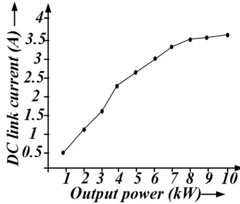
Fig. 7.4. DC link current vs output power level
