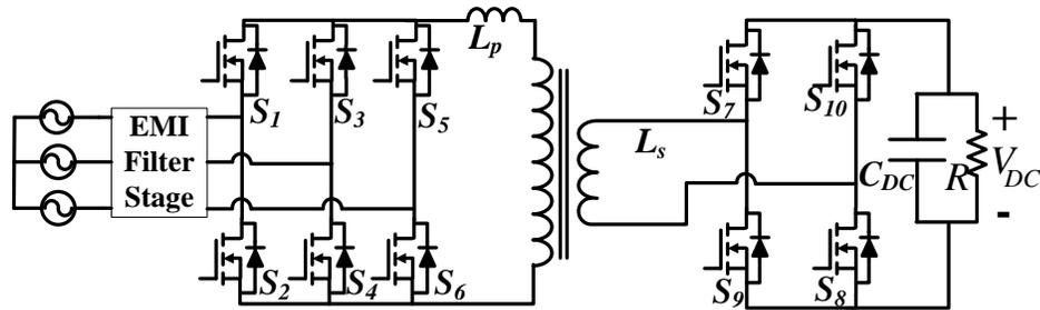
Fig. 8. 2. Three-phase matrix-converter based RTRU (alternative-2)
