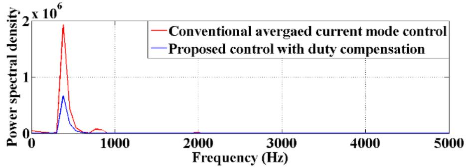
Fig. 2.7. FFT plot of the phase ‘A’ current at two different control methods
