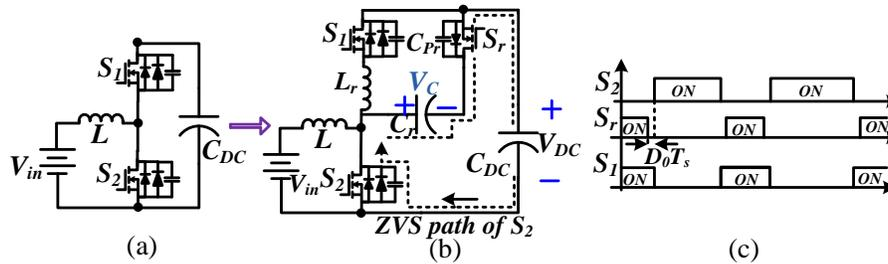
Fig. 2.16. ZVS active clamping in a regular DC-DC boost converter
