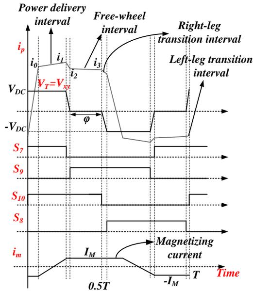
Fig. 6. 16. Typical waveforms of primary voltage, primary current and the gate pulses in a PSFB converter.
