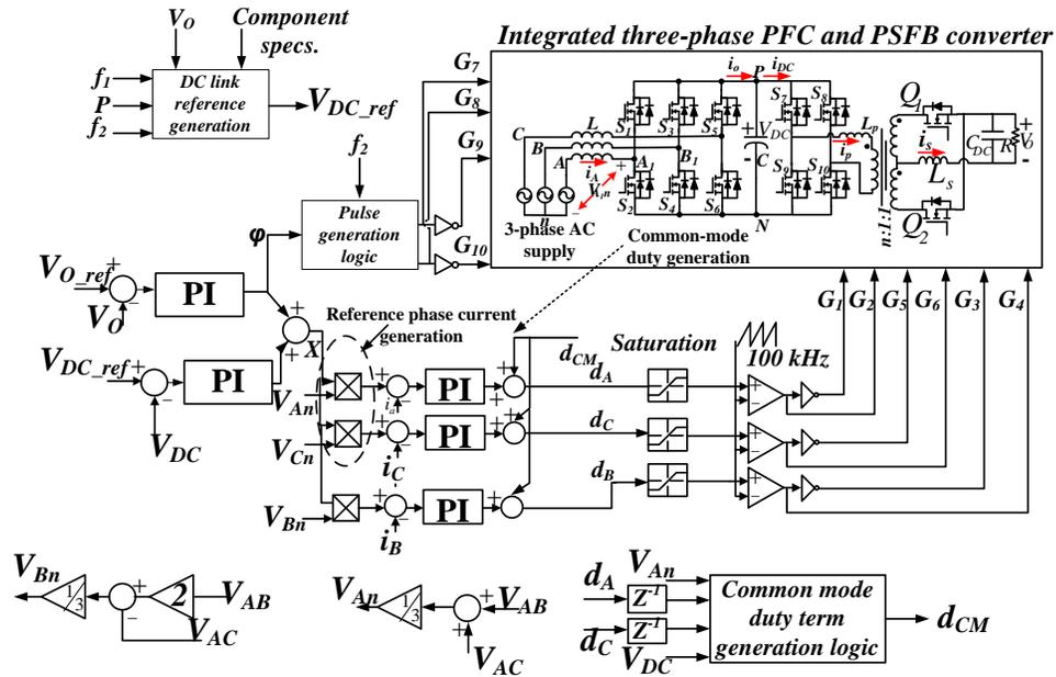
Fig. 6. 21. Variable DC link control method of an integrated two-staged AC-DC converter.
