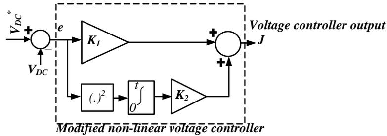
Fig. 3. 1. The proposed voltage controller
