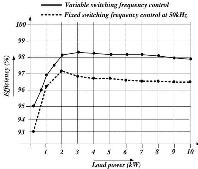
Fig. 4.14. Efficiency comparison between fixed and variable frequency control at different load power levels
