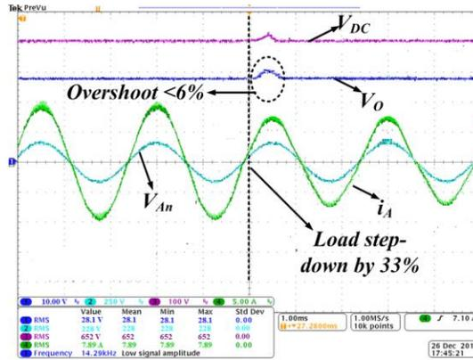
Fig. 7.17. The converter waveforms under load step-down from 6kW to 4kW
