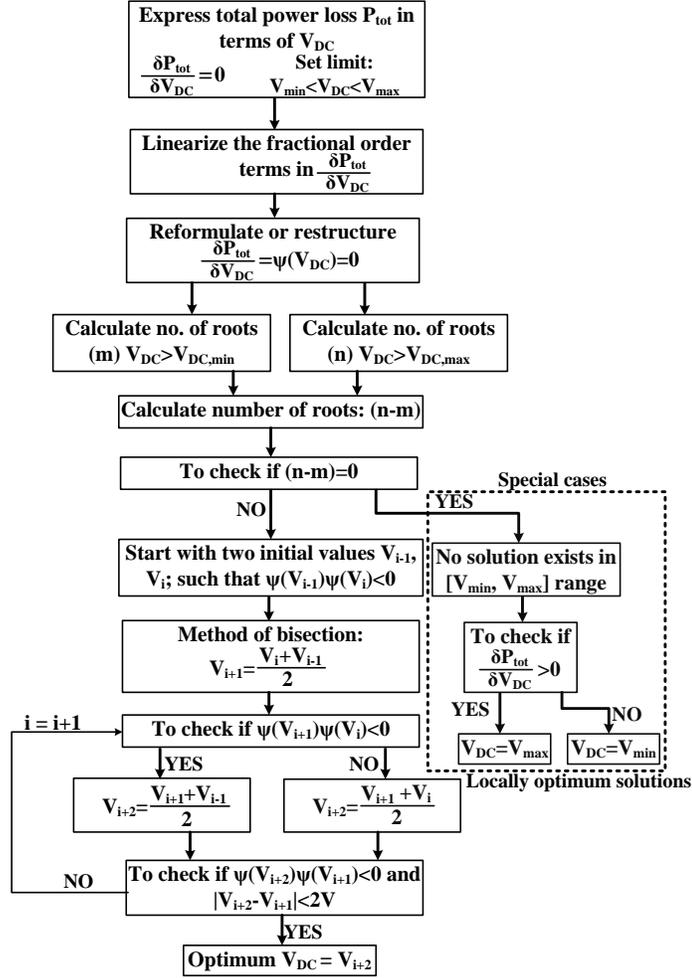
Fig. 6. 19. Flowchart of determining optimum  $V_{DC}$  by the proposed analytical method
