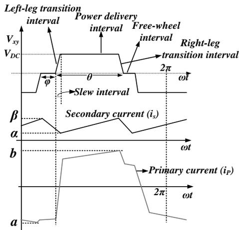
Fig. 6. 17. Typical waveforms of primary and secondary currents
