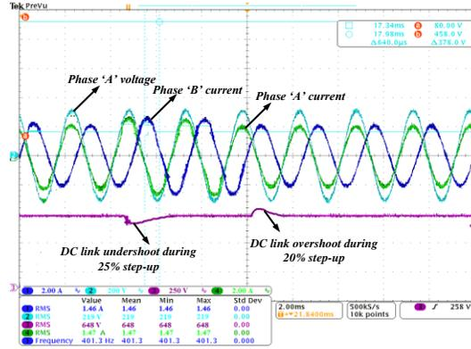
Fig. 3.16. Load transient of PFC converter from 1kW to 1.25kW and from 1.25kW to 1kW
