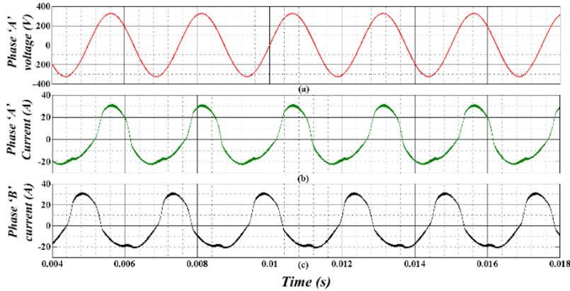
Fig. 2.5. Simulation results of three-phase boost PFC at 10kW power with averaged-current mode control (without any additional duty compensation).
