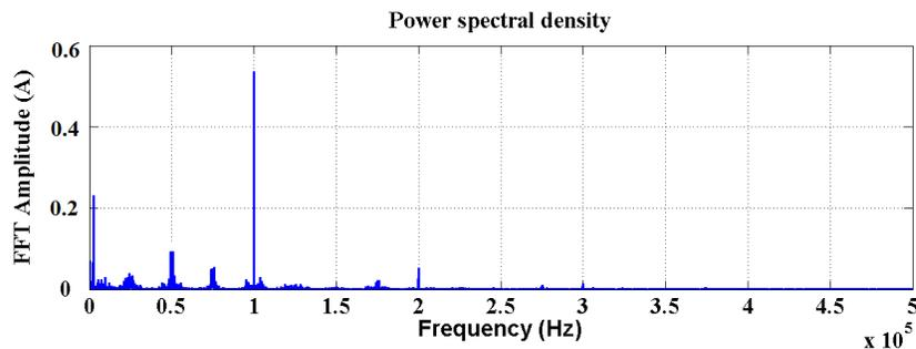
Fig. 7.9. FFT of the DC link capacitor current under the proposed control strategy
