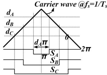
Fig. 7.3. Switching function generation
