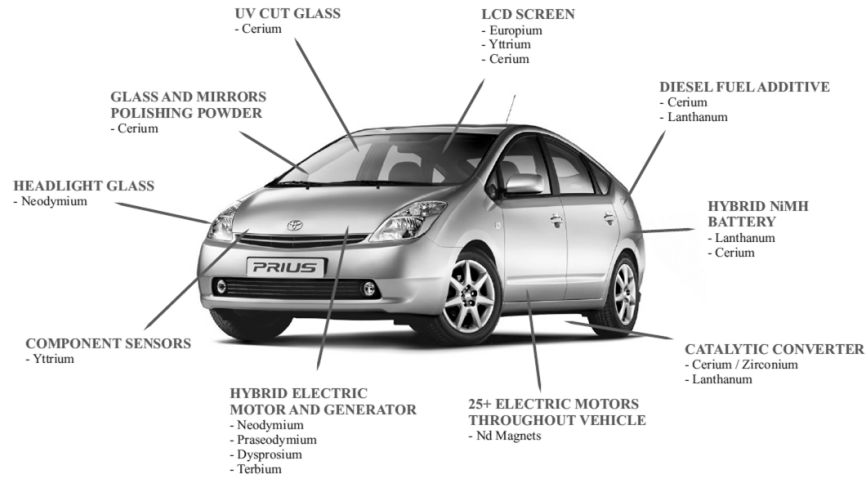
Figure 1.3: Rare Earths Used in a Hybrid Electric Vehicle (HEV) [17]
