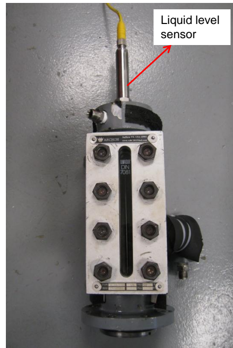
Figure 2-10: Flash tank with the liquid level sensor installed
