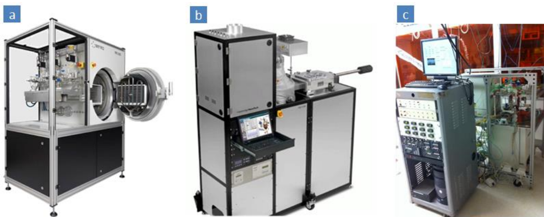
Figure A1: (a) Beneq TSF 500 ALD system for V 2 O 5 and Al 2 O 3 , (b) Cambridge Nanotech Fiji ALD system for TiN, (c) Home-made furnace system for Ru deposition.
