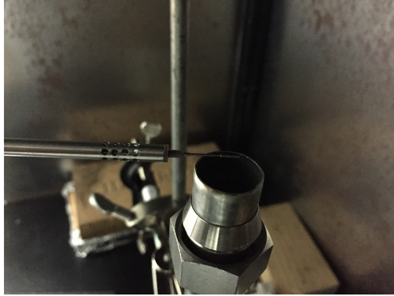
Figure 3.4: 17 mm free-jet style rig and the model 6542 OMNI probe
