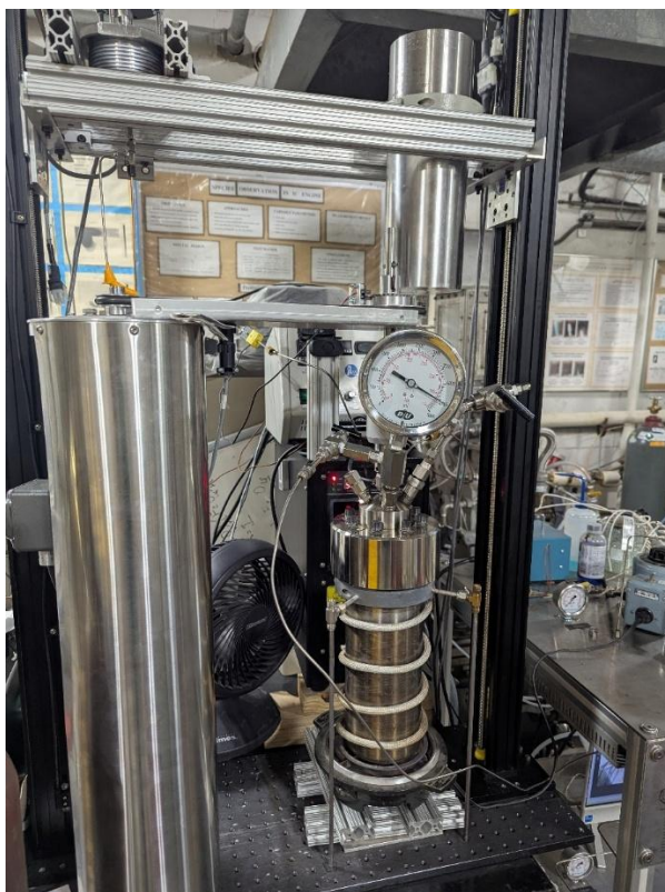
Fig. 7 Reactor with heated base plate added
