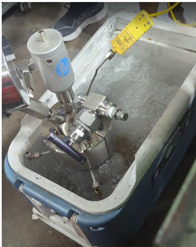
Fig. 16 Immersion cooling test using ice water bath
