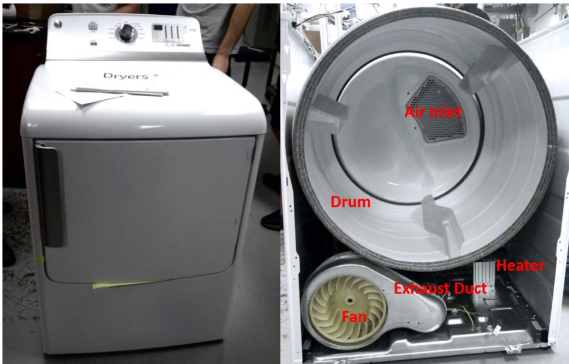
Figure 6: GE electric clothes dryer (Model number: GHDN520EDWS)
