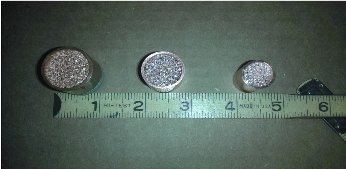
Figure 4-3: Copper foam heat exchangers in three sizes.
