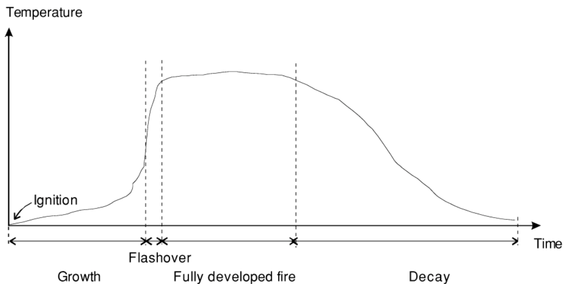
Figure 1-1: Temperature variation with time in an enclosure fire. [3]
