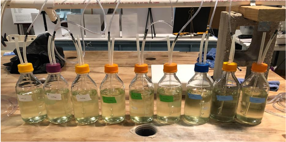
Figure 4.1 Crassostrea virginica ( C. virginica ) larval exposure to nylon 6, 6 (10 x 10 \mu\text{m} , 10 x 30 \mu\text{m} ) or polyethylene terephthalate (PET, 14 x 14 \mu\text{m} , 14 x 28 \mu\text{m} ) microfibers at 100 and 1000 fiber \text{mL}^{-1} . Larvae and all particles were kept in suspension by aeration with glass tubes.
