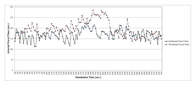
Figure 51 Observed travel time of the corridor obtained from VISSIM
