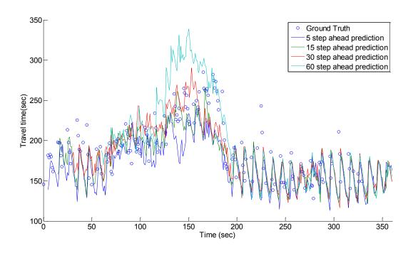
Figure 63 Westbound predicted versus ground truth travel time for 5, 15, 30 and 60 time step prediction of simulation dataset
