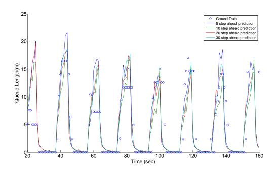
Figure 35 Predicted and ground truth queue of Peachtree street 12:45 to 1:00 cell 5
