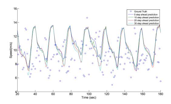
Figure 41 Predicted and ground truth speed of Peachtree street 4:00 to 4:15 cell 3
