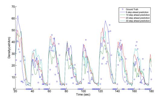
Figure 38 Predicted and ground truth queue of Peachtree street 4:00 to 4:15 cell 5
