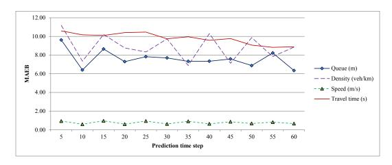
Figure 60 Line plot of average prediction MAEB of different traffic state variables of simulation dataset
