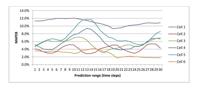
Figure 28 Plots of predicted speed MAPEB over different prediction range with NGSIM Peachtree data from 12:45 to 1:00
