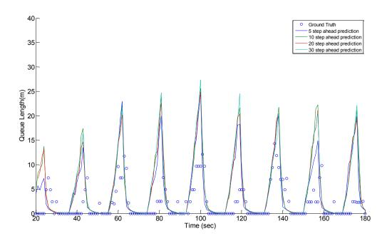
Figure 34 Predicted and ground truth queue of Peachtree street 12:45 to 1:00 cell 1
