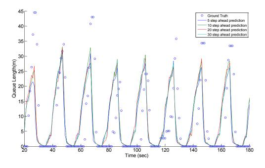
Figure 36 Predicted and ground truth queue of Peachtree street 4:00 to 4:15 cell 5
