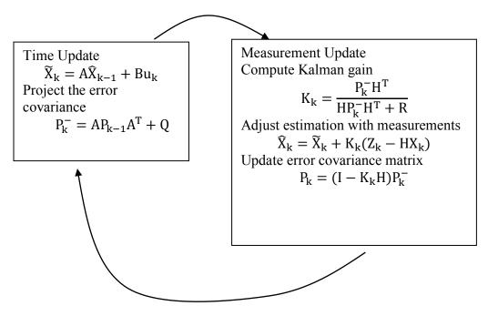
Figure 6 Computation step of KF
