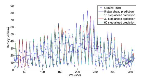
Figure 66 Predicted versus ground truth density of cell 2 of simulation dataset
