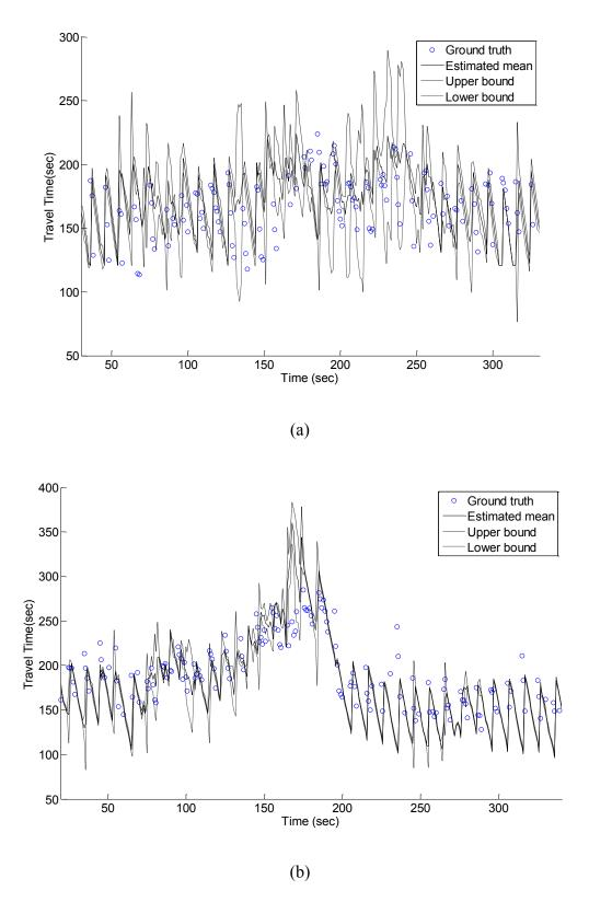
Figure 56 Estimated versus ground truth travel time plot of (a) Eastbound traffic (b) Westbound traffic of simulation dataset
