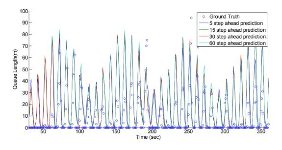
Figure 64 Predicted versus ground truth queue length of cell 8 of simulation dataset
