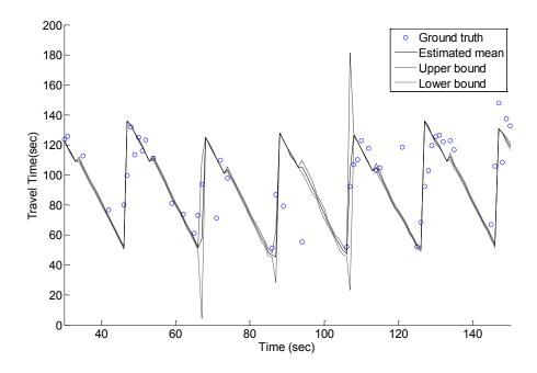
Figure 18 Estimated and ground truth travel time of PT street 4:00 to 4:15 northbound traffic
