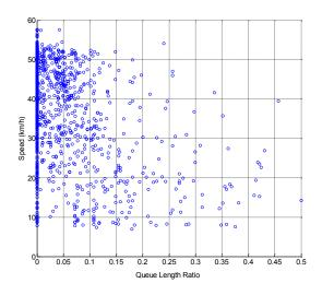
Figure 53 Observed speed and queue ratio plot of (a) Eastbound traffic (b) Westbound traffic of simulated network
