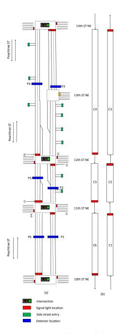
Figure 11 The sketch of geometric layout of the Peachtree arterial and corresponding cell network structure
