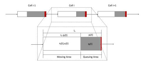
Figure 2 Illustration of moving and queuing area within a cell
