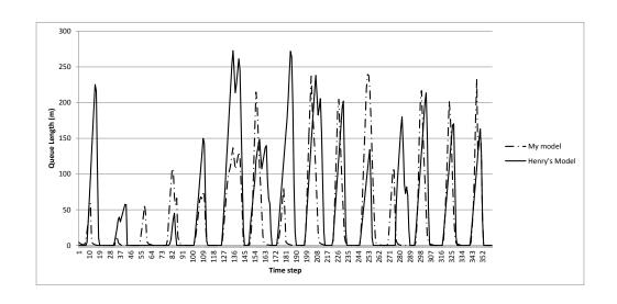
Figure 45 Comparison of estimated queue length of cell 1
