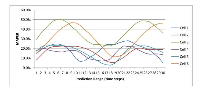
Figure 25 Plots of predicted queue length MAPEB over different prediction range with NGSIM Peachtree data from 4:00 to 4:15
