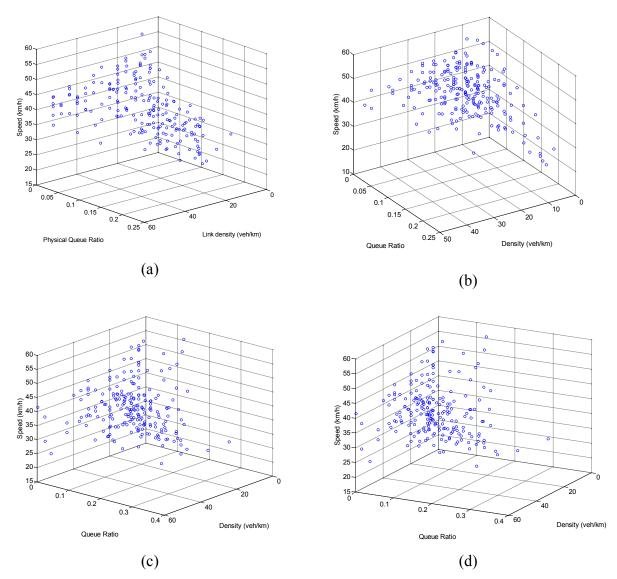
Figure 15 (a) ~ (d) The speed-density-queue three dimensional scatter plots of Peachtree street
