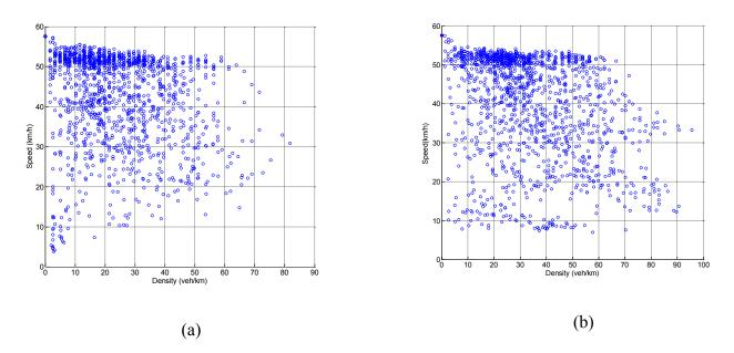
Figure 52 Observed speed and density plot of (a) Eastbound traffic (b) Westbound traffic of the simulated network
