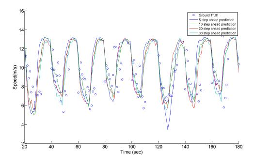
Figure 42 Predicted and ground truth speed of Peachtree street 4:00 to 4:15 cell 5
