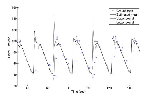
Figure 17 Estimated and ground truth travel time of PT street 12:45 to 1:00 southbound traffic
