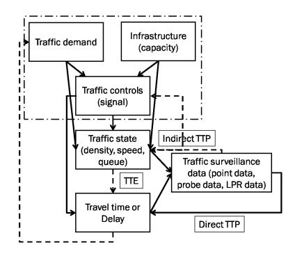
Figure 8 Relationship between traffic state, travel time and traffic surveillance data
