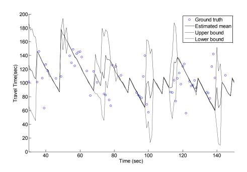
Figure 19 Estimated and ground truth travel time of PT street 4:00 to 4:15 southbound traffic
