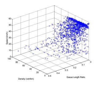
Figure 54 Observed speed, density and queue ratio 3-D plot of (a) Eastbound traffic (b) Westbound traffic of simulated network
