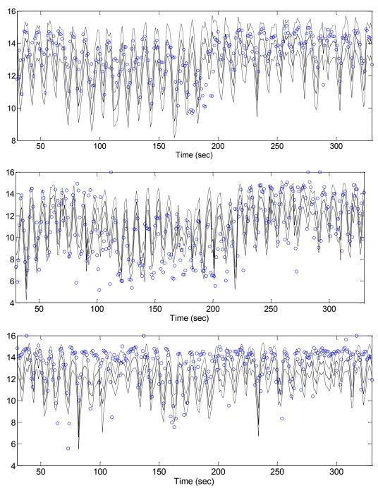
Figure 59 Estimated versus ground truth density plot of (a) Cell 5 (b) Cell 6 (c) Cell 7 of simulation dataset
