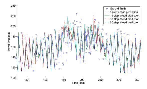
Figure 62 Eastbound predicted versus ground truth travel time for 5, 15, 30 and 60 time step prediction of simulation dataset
