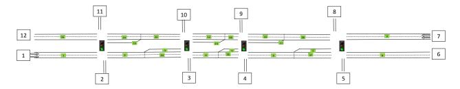
Figure 50 Number of demand generation and sink nodes of the simulation network
