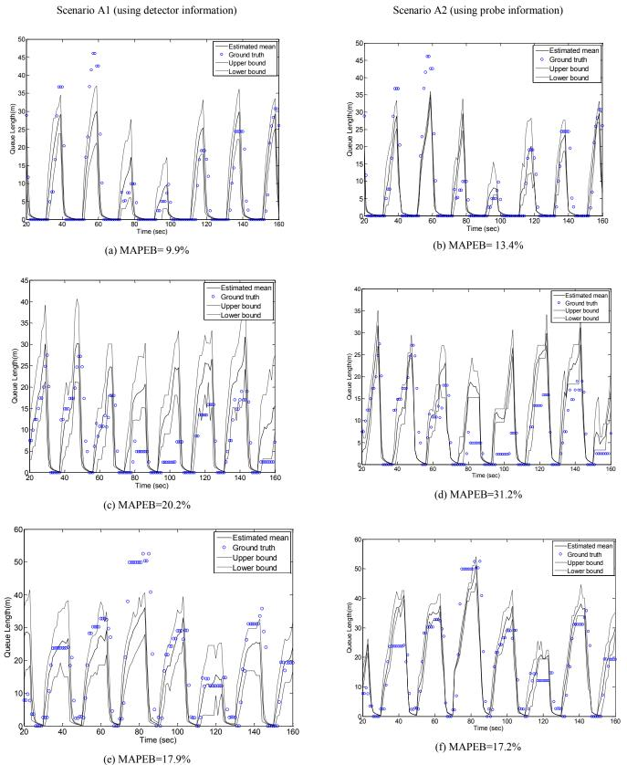
Figure 20 Estimated and ground truth queue length plot of selected cells in NGSIM dataset
