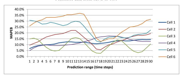
Figure 27 Plots of predicted density MAPEB over different prediction range with NGSIM Peachtree data from 4:00 to 4:15
