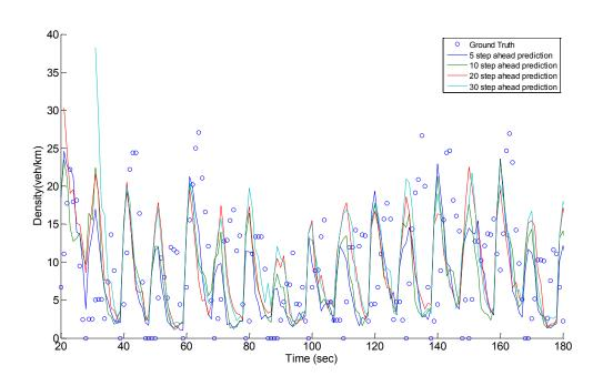
Figure 37 Predicted and ground truth queue of Peachtree street 4:00 to 4:15 cell 6
