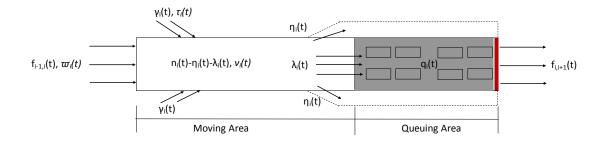
During interval t, the composition of the traffic flow in the moving area will change due to the traffic flows moving inbound and outbound. At the beginning of interval t+1, the moving area contains three groups of vehicles. The first group is the vehicles remaining
