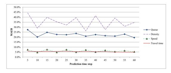
Figure 61 Line plot of average prediction MAPEB of different traffic state variables of simulation dataset
