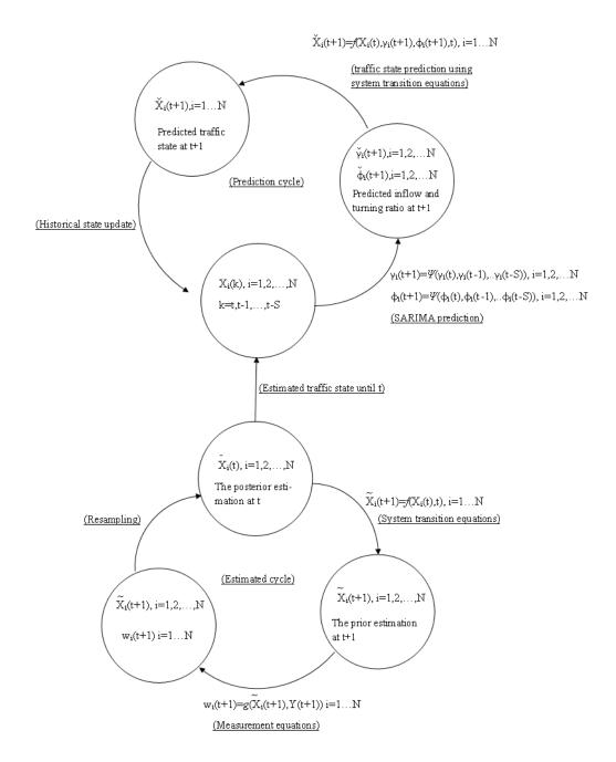
Figure 9 Real-time traffic state estimation and short-term prediction flow chart
