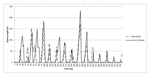
Figure 48 Comparison of estimated queue length of cell 4
