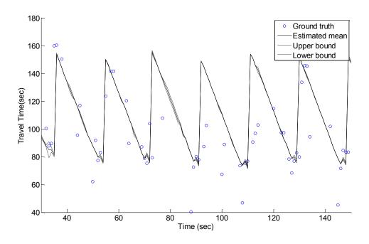
Figure 16 Estimated and ground truth travel time of PT street 12:45 to 1:00 northbound traffic
