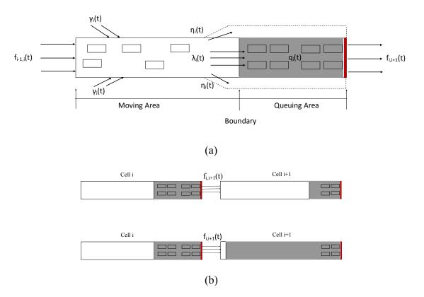
Figure 3 Traffic flow movements inside a cell (a) and traffic flow between two adjacent cells (b)
