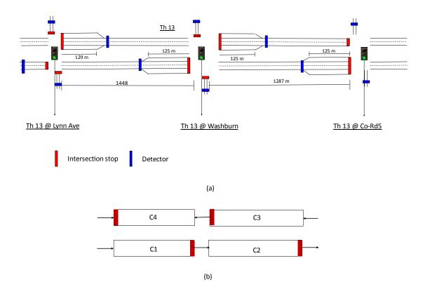
Figure 44 Geometric layout (a) and cell network structure (b) used in comparison study
